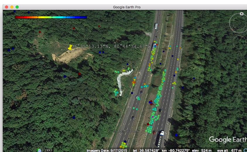
(a) The location of the soil slope (the yellow pin) near MP1.8. The color of the points is the estimated velocity from  $-10$  to  $10$  mm/yr.
