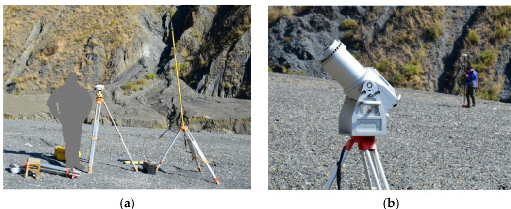
**Figure 5.** Ground LiDAR survey in the Jiangjia Gully area showing (a) DGPS base station (b) RIEGL Z-6200 laser scanner.
