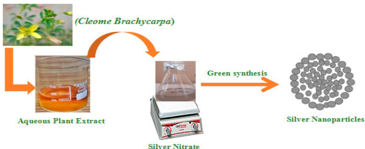
**Scheme 2.** Schematic diagram for biological synthesis of AgNPs.
