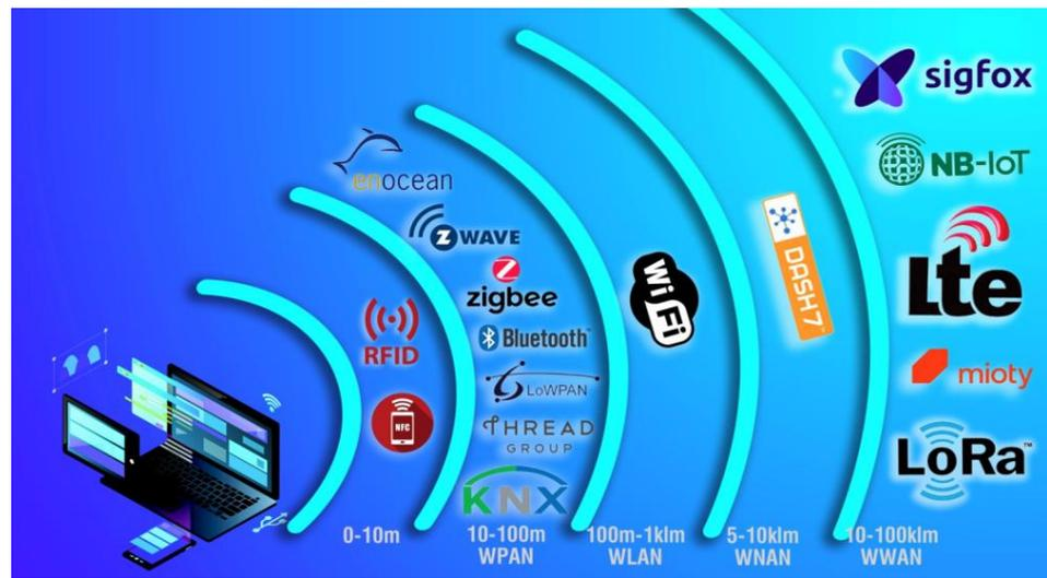
**Figure 4.** Illustration of existing technologies for wireless networking regarding connectivity range.
