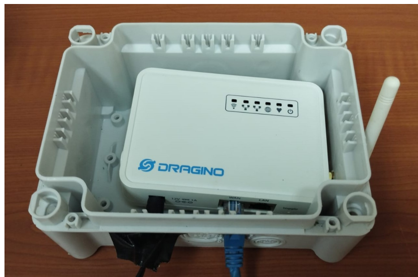
Figure 4. LoRaWAN gateway for the physical implementation.
