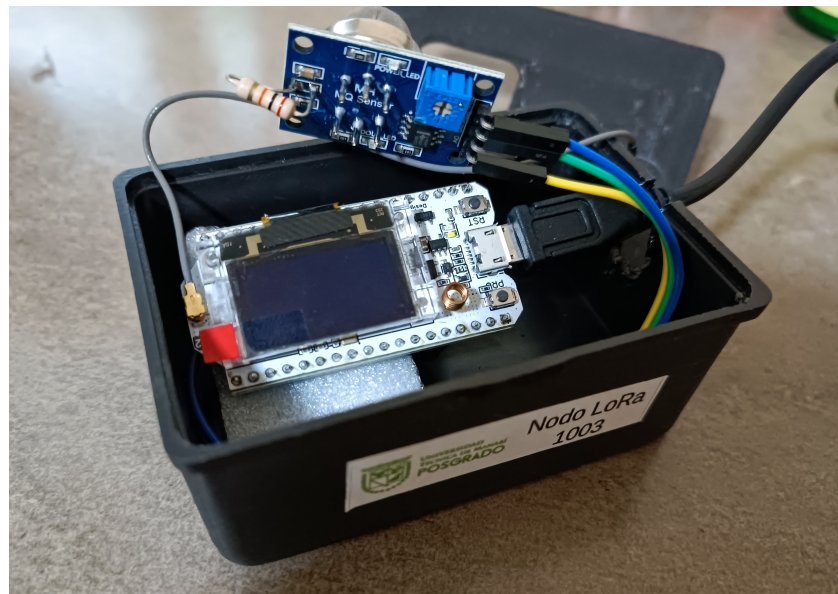
Figure 3. Sensor node used in physical implementation.
