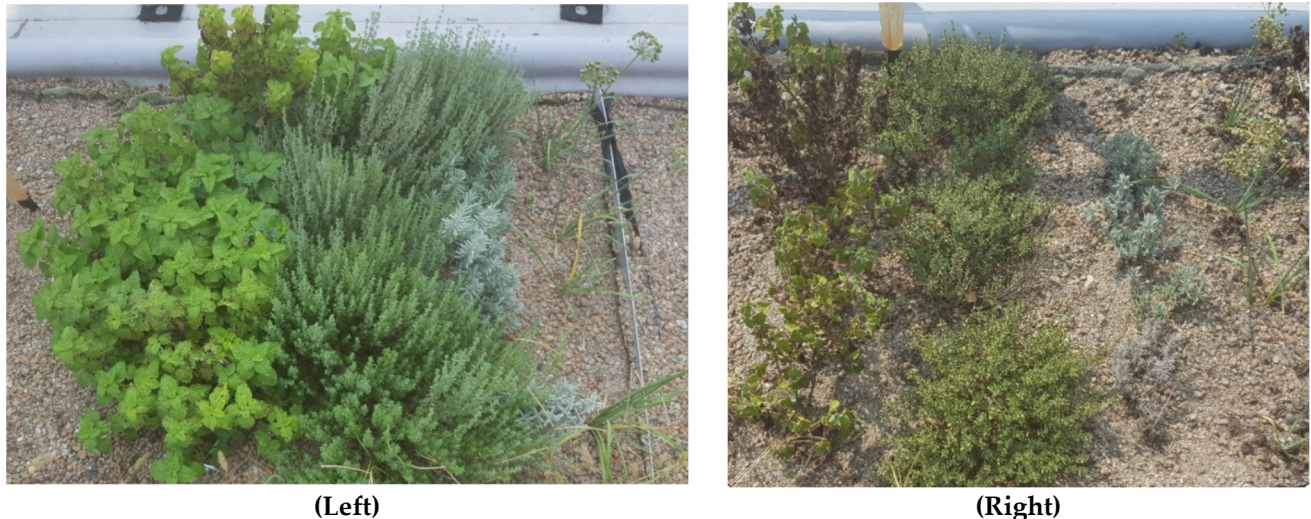
Figure 1. Comparison of watering regimes (1 L per plant) of twice per week (left) and once every two weeks (right) for the green roof perennial herb experiment.
