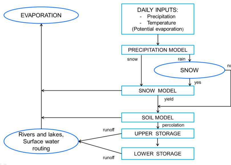
**Figure 3.** The schematic figure of the hydrological model used in Finland based on the data presented in Figure 6 originally published in Vehviläinen & Huttunen [33].
