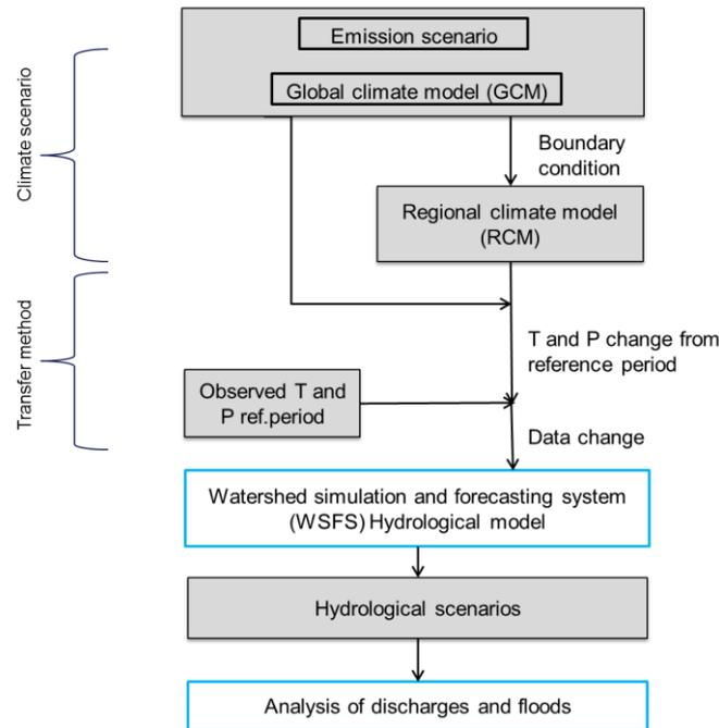
**Figure 2.** Schematic figure of the method used in flood assessment in Finland based on the data presented in Figure 11 originally published in Veijalainen *et al.* [28]. Grey boxes indicate input/output data and white boxes research methods.
