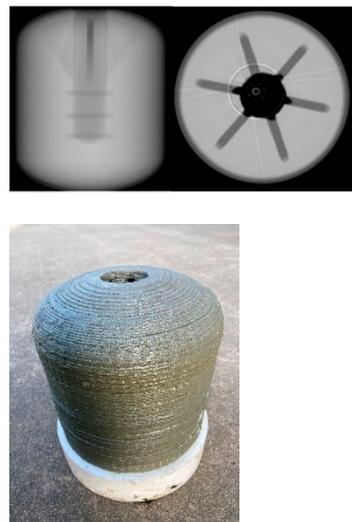
**Figure 7.** Non-destructive experiment of coated grain.
