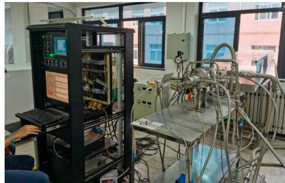
**Figure 9.** The combustion gas generator and measurement and control system of the test system.
