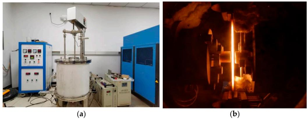
**Figure 14.** The calibration system of the Gardon heat flux meter: (a) calibration system; (b) calibration test.
