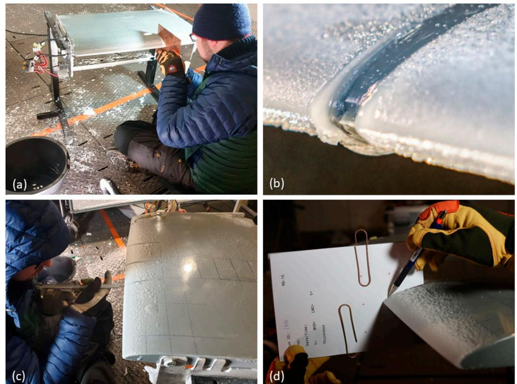
**Figure 3.** Steps of the ice accretion measurement process: (a) the iced leading edge is cut in several span-wise locations using a heated metallic plate with a negative shape of the airfoil's leading edge. Using the formed ice cuts—detailed in (b)—caliper measurements of the leading-edge ice thickness are performed (c), followed by the manual tracing of the 2D ice profile (d).
