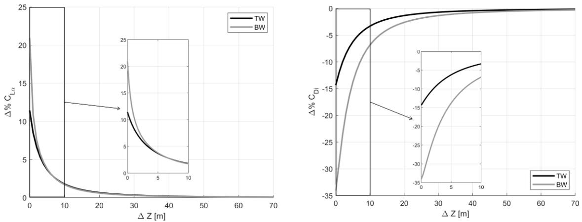
Figure 15. TW and BW IGE effects comparison:  $\Delta\%C_{L\alpha}$  (left),  $\Delta\%C_{Di}$  (right).
