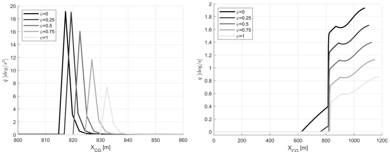
**Figure 20.** BW angular pitch acceleration (left) and angular pitch speed (right) varying  $\psi$  ( $\delta_f = 30^\circ$ ,  $V_R = 1.15V_{s\ TO}$ ).
