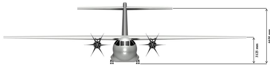
**Figure 7.** Front view of the regional HE-TW test case.
