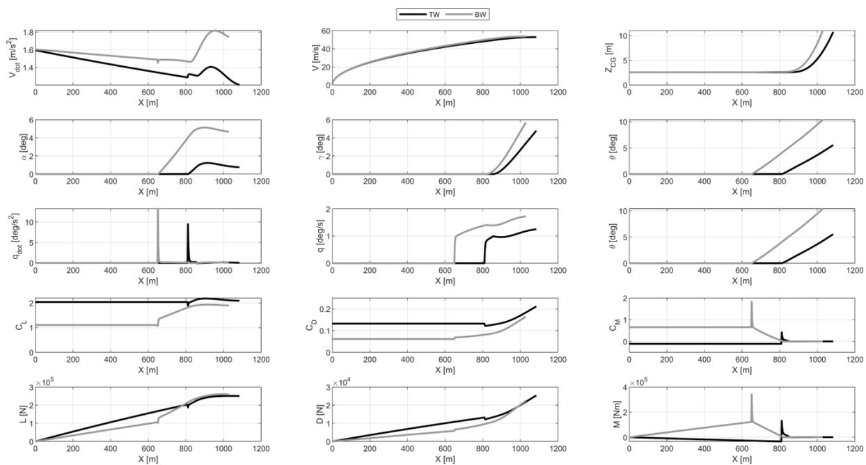
**Figure 26.** Optima TW vs. BW comparison of kinematic and aerodynamic parameters evolution during take-off.
