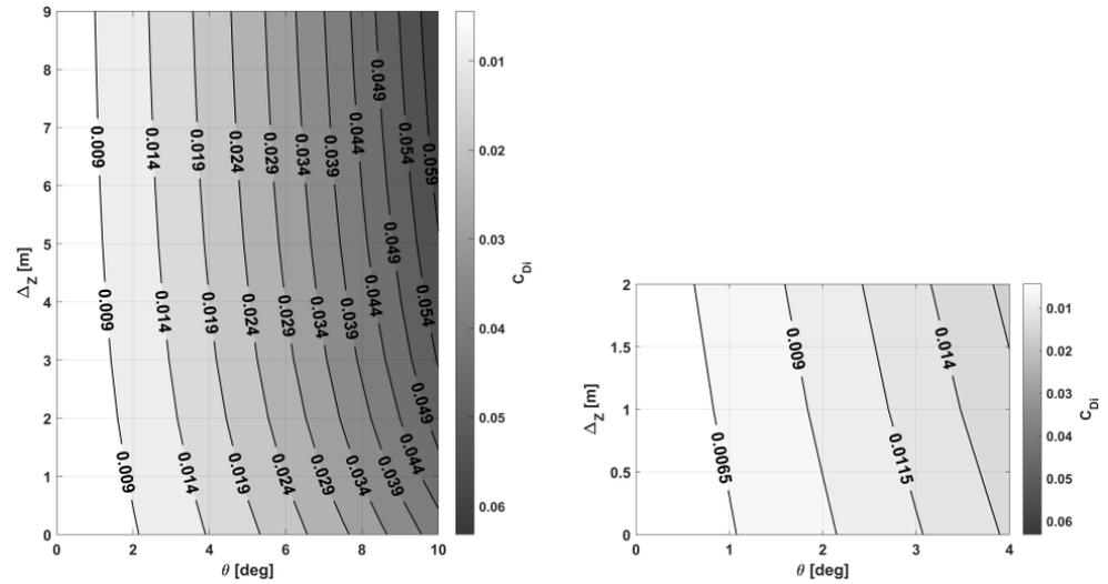
Figure 14. BW  $C_{Di}$  in ground effect varying height and pitch attitude.
