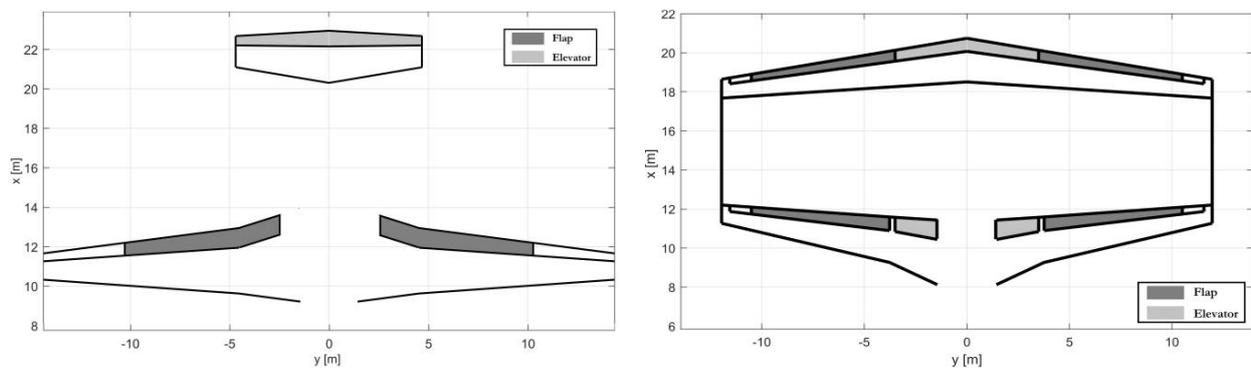
**Figure 11.** Sketch of planforms with of elevator and flaps for TW (left) and BW (right).
