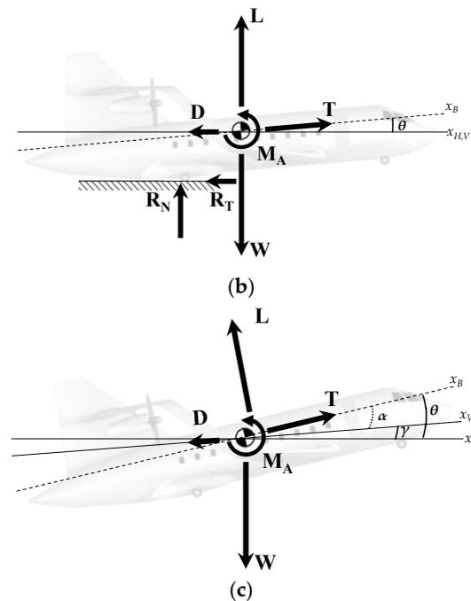
**Figure 4.** Forces schematic representation for the take-off phases: (a) ground-roll; (b) rotation; (c) transition to climb.
