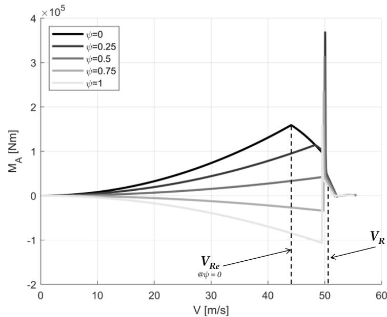
Figure 23. BW aerodynamic moment vs. take-off speed.
