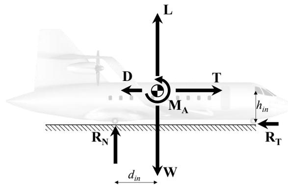
Figure 21. Simplified ground-roll forces schema.
