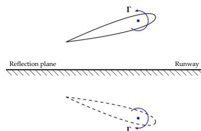
**Figure 5.** Mirroring approach for ground effect aerodynamics evaluations.
