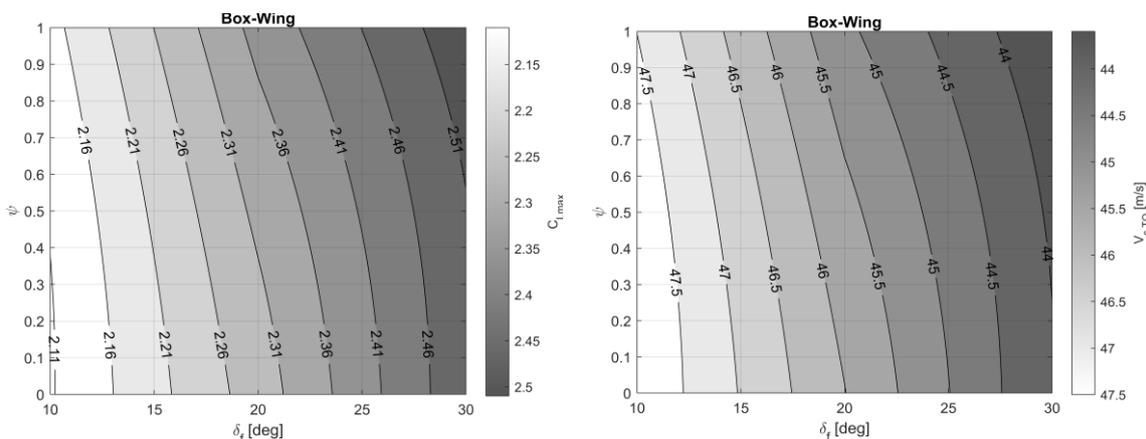
Figure 17. BW high-lift performance as a function of  $\delta_f$  and  $\psi$ :  $C_{Lmax}$  (left) and  $V_{s\ TO}$  (right).
