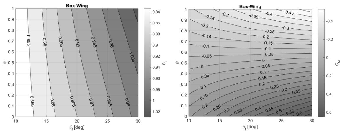
**Figure 18.** BW high-lift aerodynamic coefficients as a function of  $\delta_f$  and  $\psi$ :  $C_L$  (left) and  $C_M$  (right).
