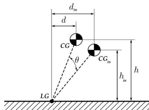
Figure 2. Centre of gravity (CG) position with respect to the main landing gear (LG).
