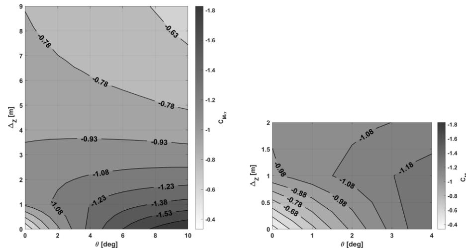
Figure 13. BW  $C_{M\alpha}$  in ground effect varying height and pitch attitude.
