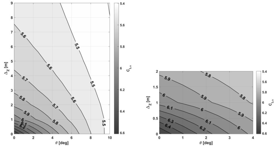
Figure 12. BW  $C_{L\alpha}$  in ground effect varying height and pitch attitude.
