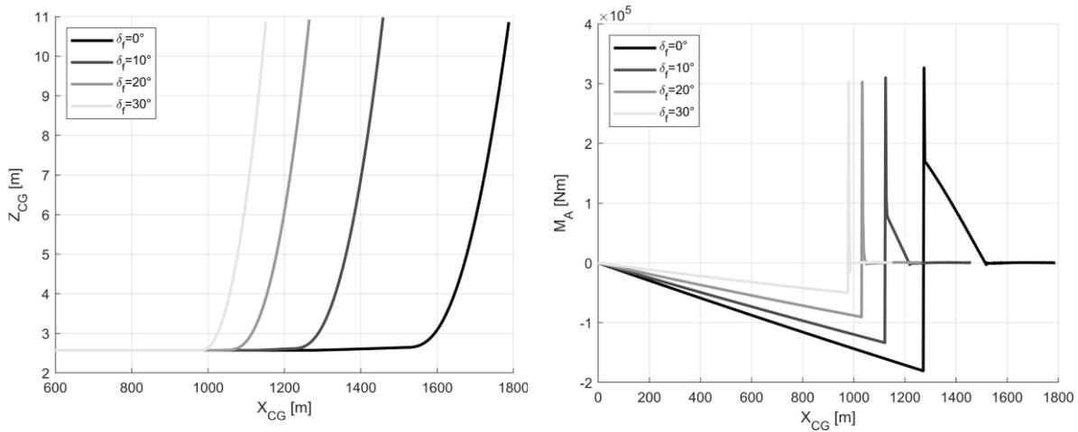
Figure 25. TW take-off trajectory (left) and aerodynamic moment (right) varying  $\delta_f$ .
