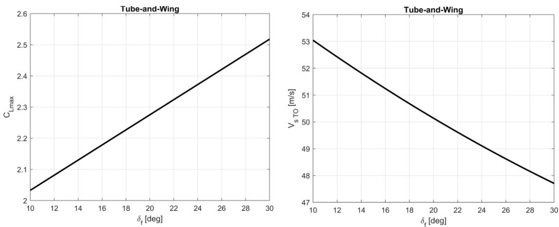
Figure 24. TW high-lift performance as a function of  $\delta_f$ :  $C_{Lmax}$  (left) and  $V_{s TO}$  (right).
