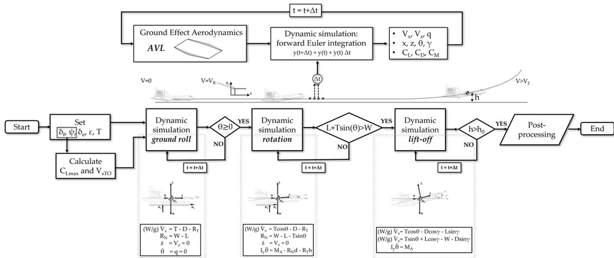
**Figure A1.** General schematic representation of the take-off simulation framework.
