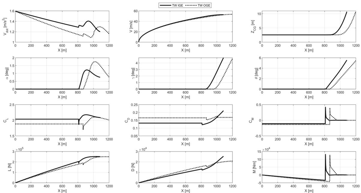
Figure 28. IGE vs. OGE comparison of TW kinematic and aerodynamic parameters evolution during take-off.
