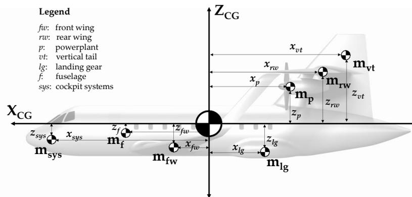
Figure 3. Simplified concentrated mass scheme of the aircraft.
