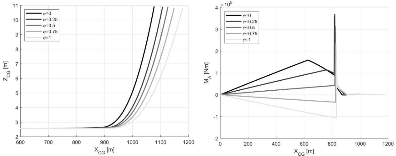
**Figure 19.** BW take-off trajectory (left) and aerodynamic moment (right) varying  $\psi$  ( $\delta_f = 30^\circ$ ,  $V_R = 1.15V_{s\ TO}$ ).
