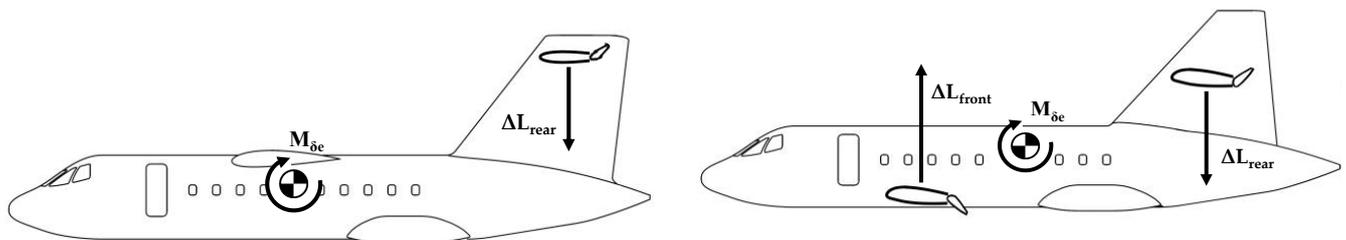
**Figure 10.** Pitch control strategies with elevator deflection for TW (left) and BW (right).
