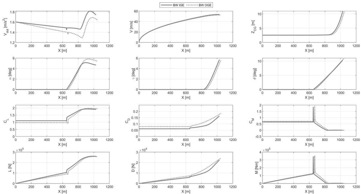
Figure 27. IGE vs. OGE comparison of BW kinematic and aerodynamic parameters evolution during take-off.
