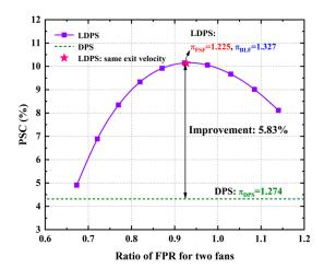
**Figure 9.** The PSC of LDPS as a function of the ratio of FPR for two fans (the PSC of DPS is displayed in green dashed line).
