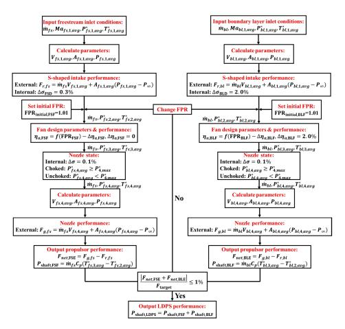
**Figure 8.** The 1D engine model and the thrust matching procedure of LDPS (the left side is the FSE model and the right side is the BLE model).
