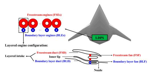
Figure 4. Concept and configuration of LDPS.
