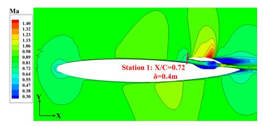
**Figure 6.** Ma contour on symmetry plane of BWB-350 with DPS at cruise (flight height of 11,000 m,  $Ma_{\infty} = 0.85$ , angle of attack of  $2^{\circ}$ ).
