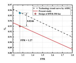
Figure 7. Fan design adiabatic efficiency as a function of design FPR by ASDL [33].
