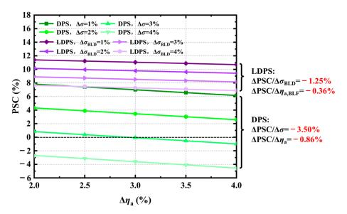
Figure 16. Comparison of the PSC of LDPS and DPS with various component performance penalties.
