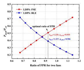
Figure 10. Normalized fan-shaft power of FSE and BLE as a function of the ratio of FPR for two fans.
