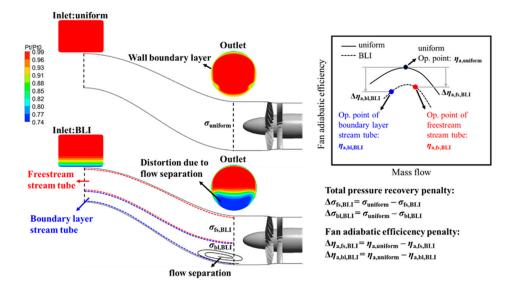
**Figure 3.** Schematic showing of the performance penalty of the S shaped and fan under uniform and BLI inlet conditions.
