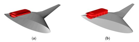
**Figure 5.** BWB-350 with different propulsion system configurations. **(a)** BWB-350 with DPS. **(b)** BWB-350 with LDPS.
