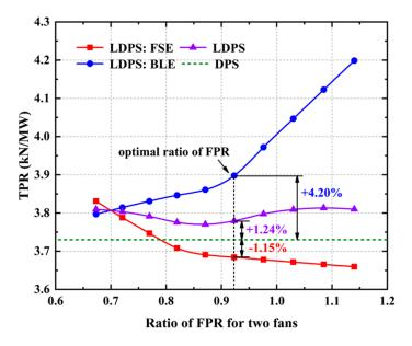
Figure 13. The TPR of FSE and BLE of LDPS as a function of the ratio of FPR for two fans.
