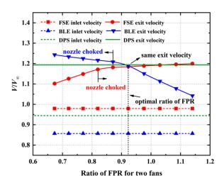
**Figure 11.** Normalized inlet and exit velocities of FSE and BLE as a function of the ratio of FPR for two fans.
