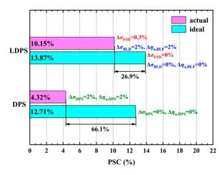
Figure 14. Comparison of the PSC of LDPS and DPS under actual and ideal conditions.
