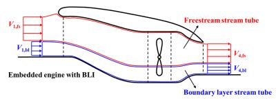
**Figure 2.** Schematic showing of flow passing through an ideal embedded engine with BLI (the freestream and boundary layer are divided into two stream tubes).
