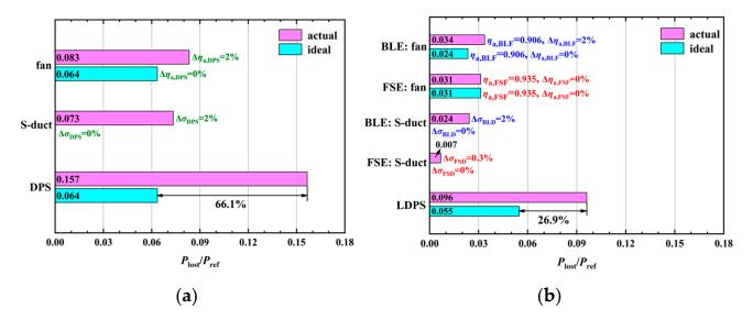
**Figure 15.** Comparison of normalized lost power of each component of LDPS and DPS under actual and ideal conditions. (a) Normalized lost power of DPS. (b) Normalized lost power of LDPS.
