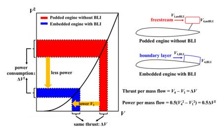
**Figure 1.** Physical principle of power-saving benefit of BLI (the ranges on the horizontal and vertical axes represent momentum and energy changes of flow passing through the engine, respectively).
