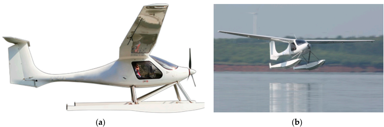
Figure 7. Experimental prototype of the RX1E-S electric seaplane. (a) Experimental prototype model; (b) prototype flight test.
