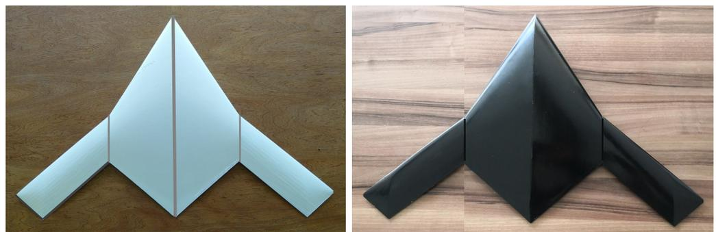
**Figure 8.** 3D-printed model (left) and surface finished and painted model (right).
