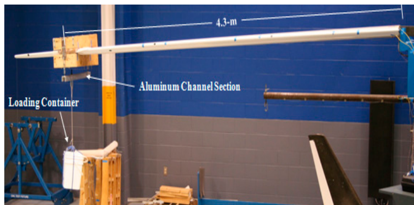
Figure 6. Concentrated load test of composite wing.
