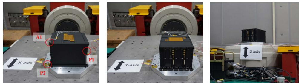
Figure 13. Vibration test configuration and accelerometer position of HSDRU.
