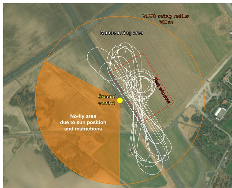
**Figure 9.** Example of SFT at level 2 using the concept of test-window and flexible pattern. This specific flight of the GFF demonstrator corresponds to the manoeuvres and performance data shown in Figure 6.
