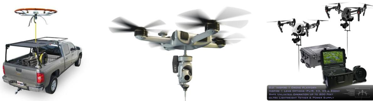
**Figure 2.** Tethered multicopters and tethered flight system for multicopters: T-Rotor [13], Hover Mast [14], Power Line [15].
