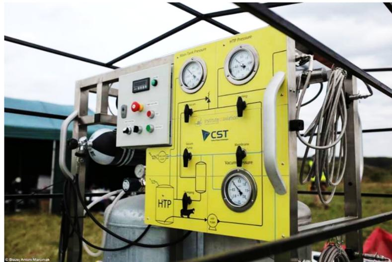
Figure 11. Mobile HTP loading station.
