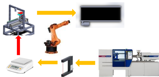
Figure 7. The handling and measurement procedure of the injection-molded part.
