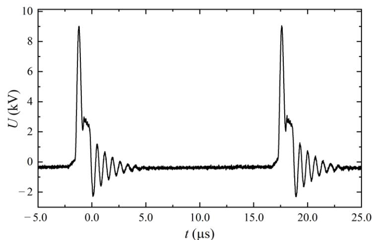
**Figure 2.** Waveform of the voltage at the HV electrode in the case of the bubble discharge.
