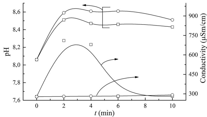
**Figure 4.** Time behavior of the pH-index and conductivity in ground water: barrier discharge (□); bubble discharge (○).
