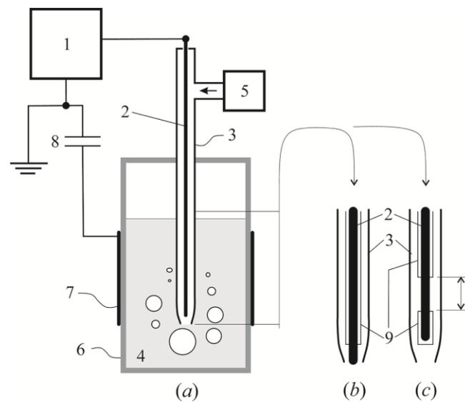
**Figure 1.** Block diagram of the experimental setup: general view (a) and zoomed sketches (indicated by arrows) of two design options of the high-voltage part (b,c). 1—power supply; 2—high-voltage electrode; 3—air feeding tube; 4—aqueous solution; 5—membrane air pump; 6—quartz vessel; 7—foil electrode; 8—capacitor; 9—dielectric shell; (\*)—10-cm-length section freed from the dielectric shell.
