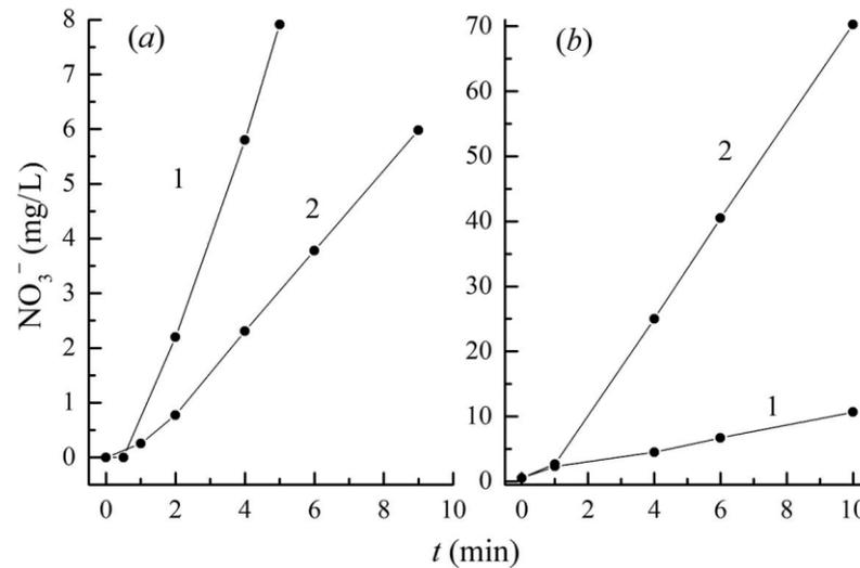
**Figure 3.** Time behavior of a specific amount of nitrate ions in distilled (a) and ground (b) water: barrier discharge (1); bubble discharge (2).
