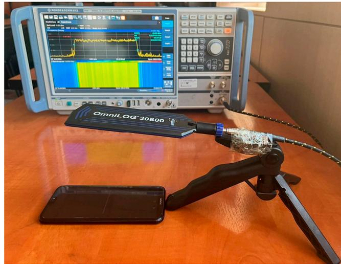
**Figure 1.** FSW spectrum analyzer, the omnidirectional receiving antenna, and the mobile phone emitting during its connection to the 5G network.
