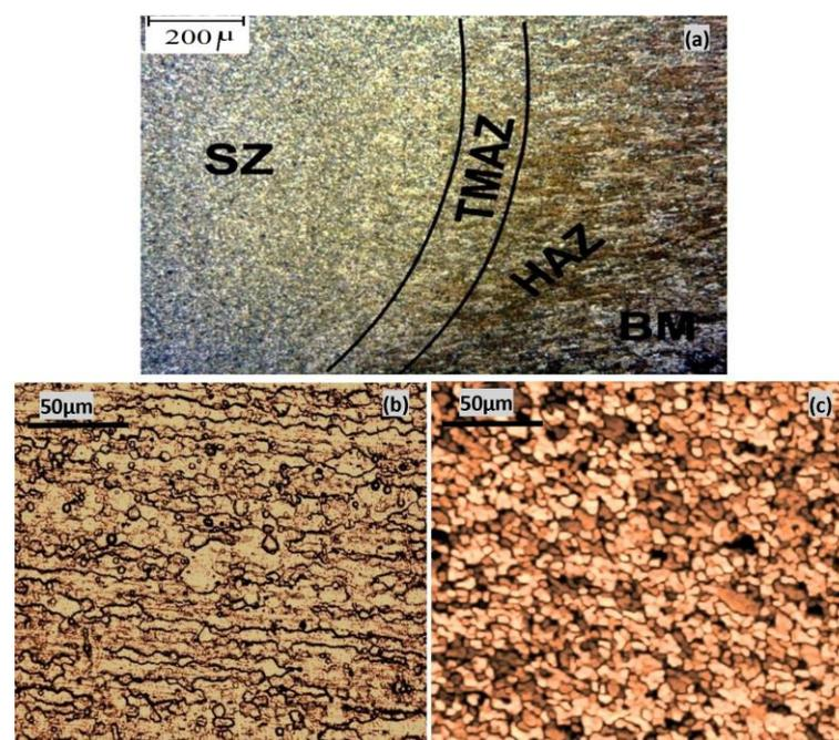
**Figure 8.** Microstructure of the grain distribution in the cross-section of the AA1100 FSW weld (processed at 1120 rpm and 250 mm/min); (a) general view of the cross-section, (b) stir zone (SZ), and (c) the base metal at higher magnification.
