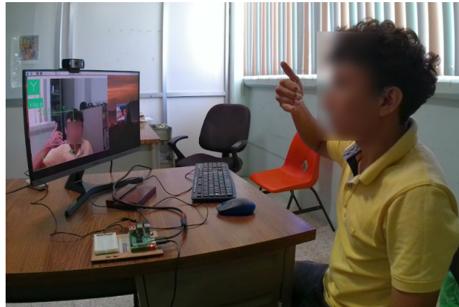
Figure 12. Implementation of the final system on the Raspberry Pi 4, with an average response time of 0.58 s.
