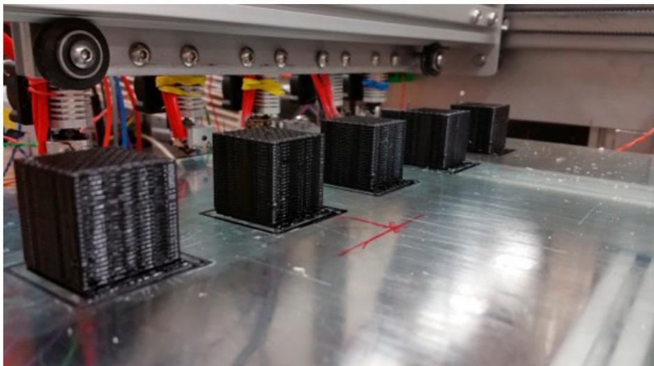
**Figure 15.** Printed component part quality (visual inspection) prior to removal from substrate to be measured for dimensional precision. As indicated in Table 9, dimensional variation between hot ends is determined to be a critical metric in contrast to print parameter adjustable deviation from nominal dimensional values (i.e., 25.4 mm).
