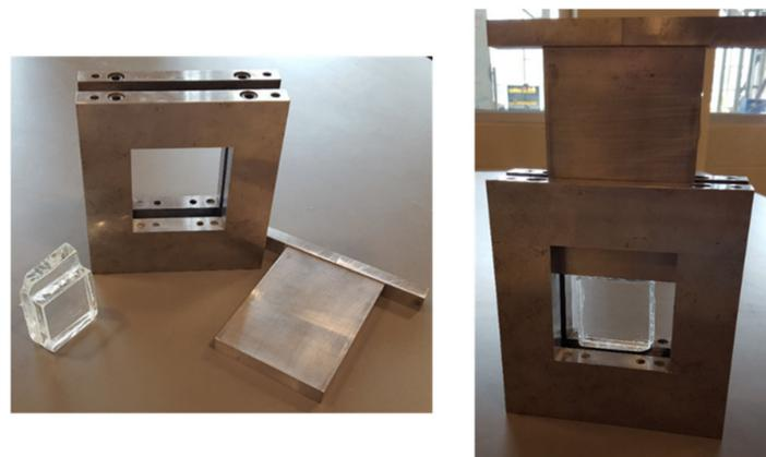
**Figure 9.** Test jig and sample for preliminary compressive load shear testing.
