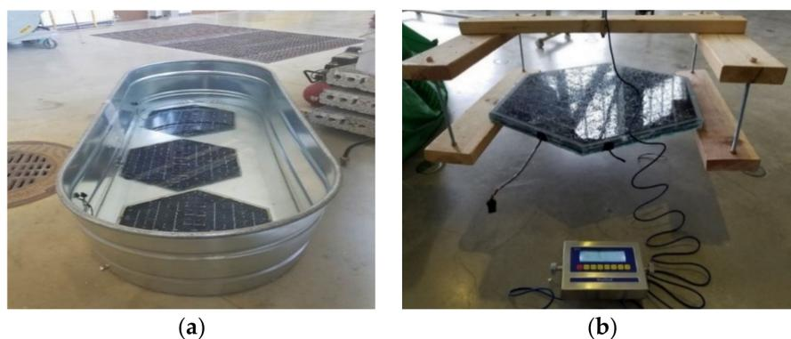
**Figure 5.** Moisture conditioning duration testing: (a) single 1135.62 liter aluminum container used during the SRP moisture conditioning duration testing. The paver electrical connectors were fixed above the waterline during testing; (b) test apparatus for weighing the solar road panels (SRPs) before and after each moisture conditioning test.
