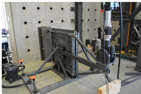
**Figure 13.** Shear test fixture with “SR3” paver installed in EMSTL.
