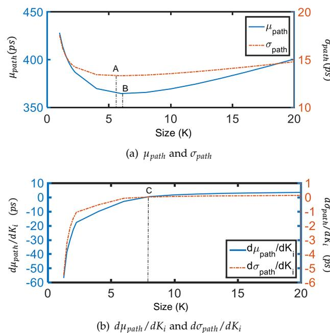
**Figure 4.** (a) Mean and standard deviation of the delay of the logic path in Figure 2 when gate  $G_i$  is sized-up; (b) derivative of the mean and standard deviation of the delay of the logic.
