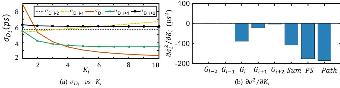
**Figure 3.** (a) changes in the delay standard deviation as gate  $G_i$  is sized-up in Figure 2; (b) changes in the delay variances as gate  $G_i$  of Figure 2 is sized-up by an amount  $\Delta K_i$ .
