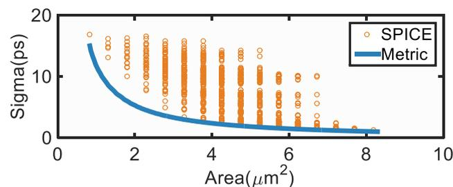
**Figure 5.** Fine metric validation with SPICE using the logic path in Figure 2
