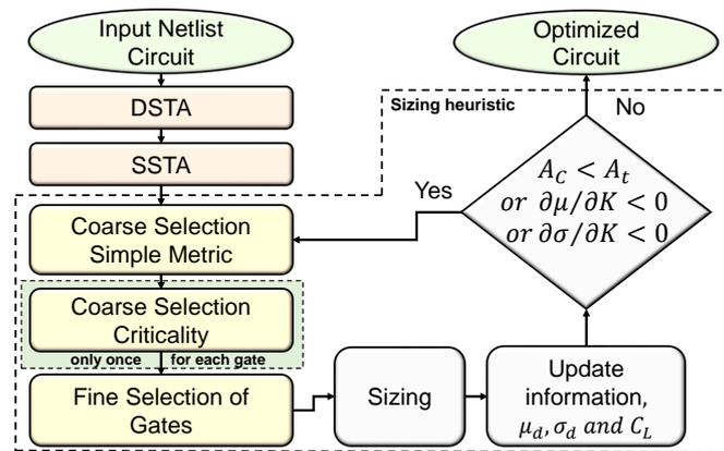
Figure 1. Flow diagram of the proposed circuit performance optimization methodology.
