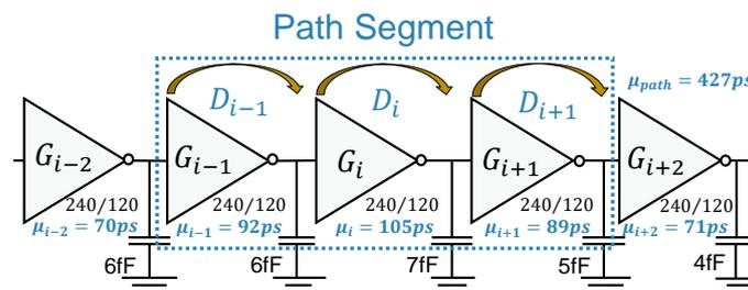
Figure 2. Logic path composed of 5-inverters.
