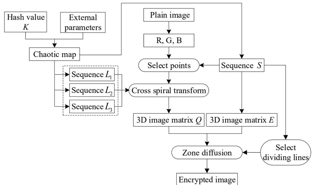
Figure 11. Block diagram of color image encryption process.
