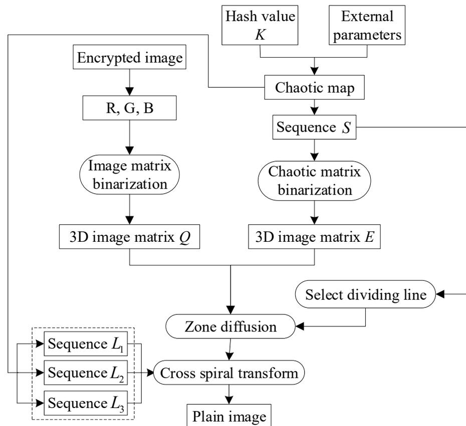
Figure 12. Block diagram of the color image decryption process.
