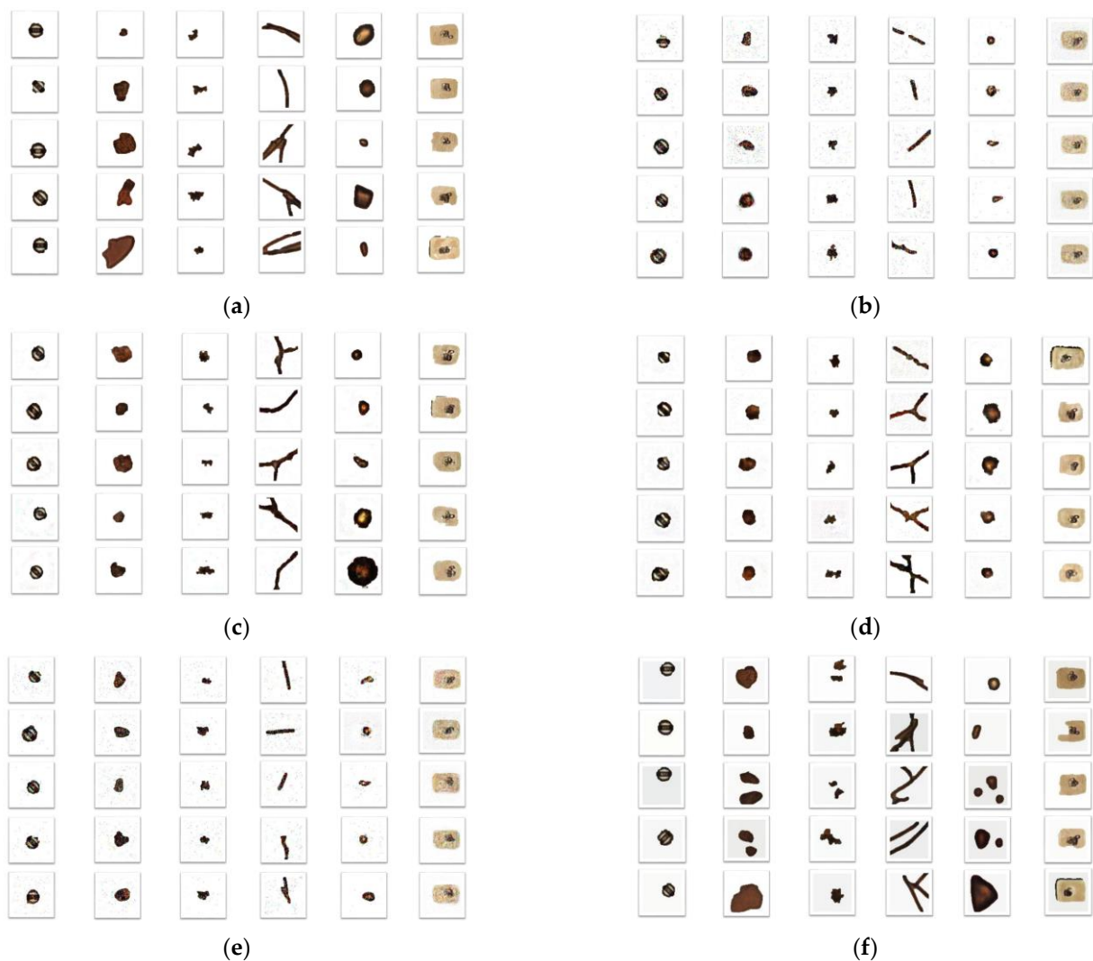
Figure 2. Defective regions for each class: (a) real images; (b) generated by vanilla GAN; (c) generated by DCGAN; (d) generated by ACGAN; (e) generated by BGAN; (f) generated by DDPM.
