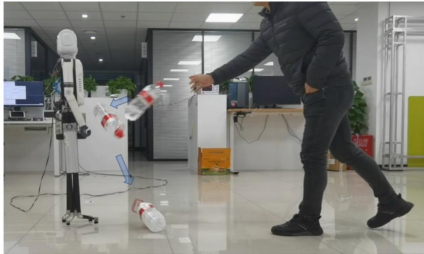
Figure 18. L04 Robot robust walking.
