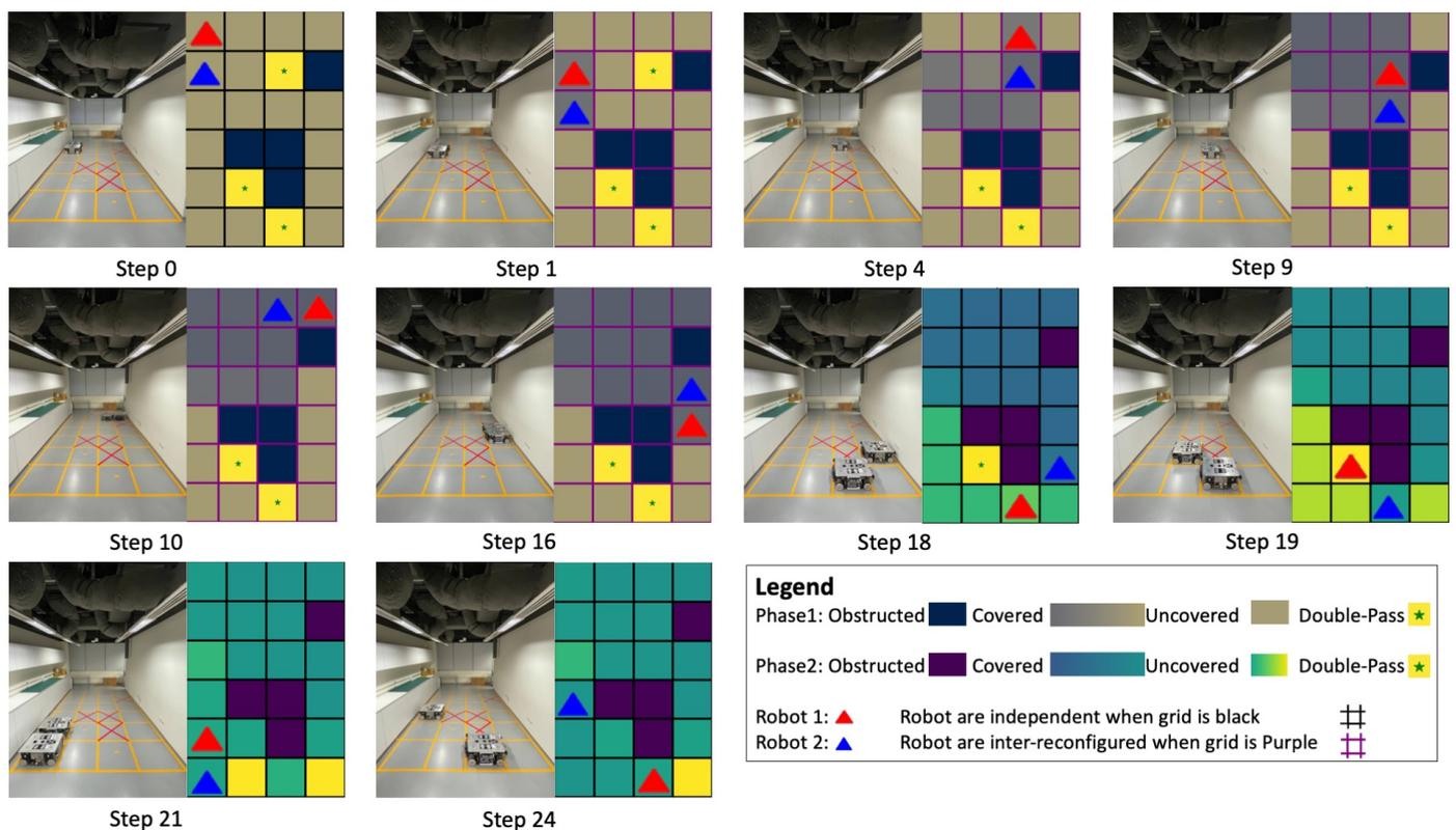
Figure 9. Simulation test environment. The robots are shown in their respective initial positions for all simulations.
