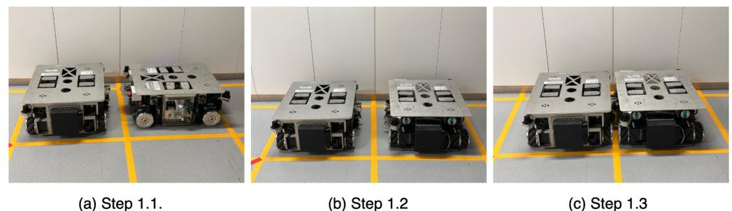
**Figure 8.** Docking process of two Wasp units into a fused state.
