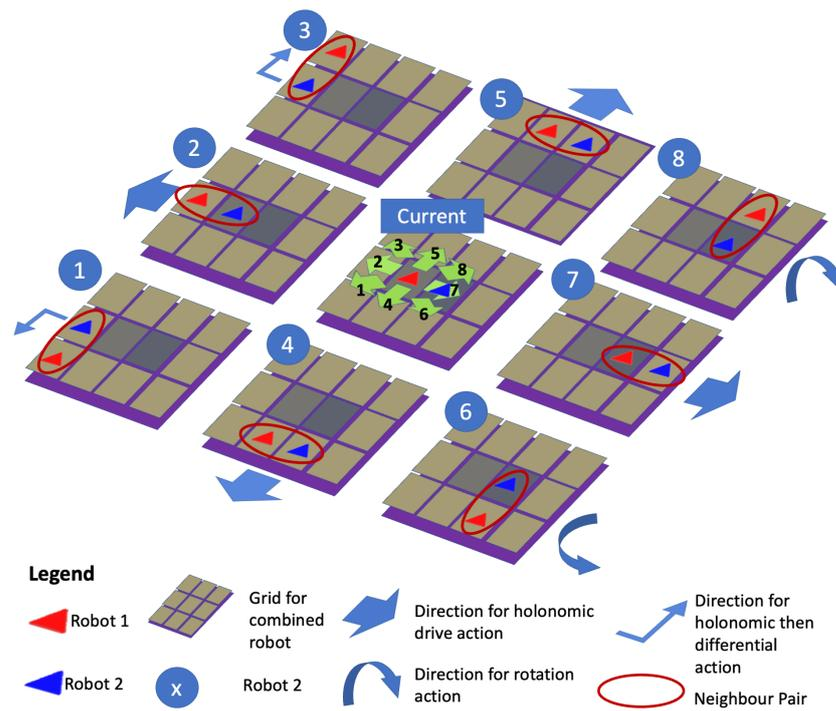
**Figure 6.** Eight possible neighbor pairs for an inter-reconfigurable robot in the fused state, containing the possible positions for  $R_1$  and  $R_2$ .
