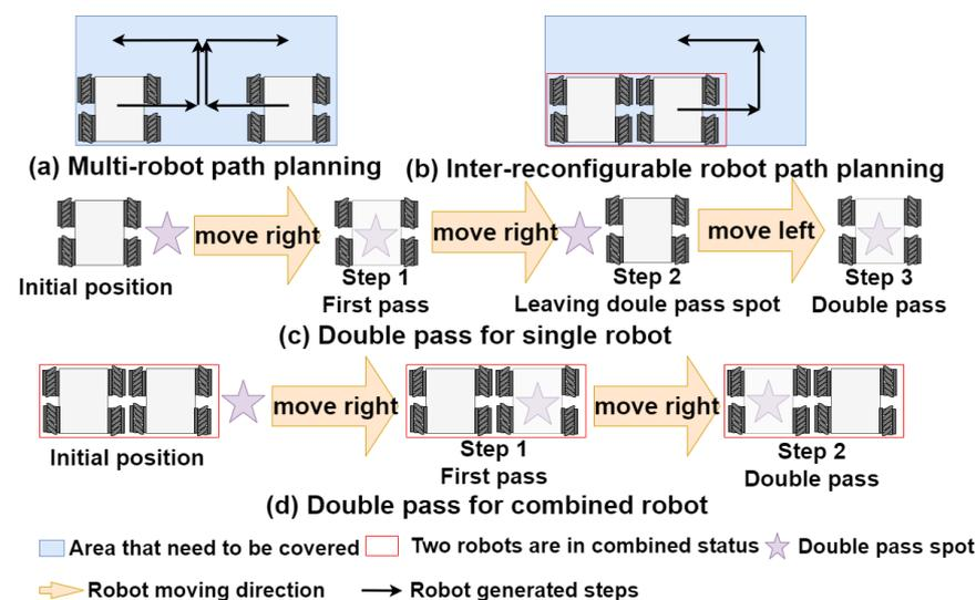
**Figure 1.** (a) A dual-robot system with its zig-zag algorithm paths. (b) The path can converge into a single path line. (c) How a single robot covers a double-pass area. (d) How a combined inter-reconfigurable robot covers a double-pass area.
