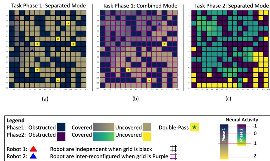
**Figure 5.** (a) GBNN [25]. (b) Proposed GBNN. (c) Phase 2. In the proposed algorithm, neural activity is  $-1$ ,  $1$ , or  $2$  when the vertex is marked as obstructed, uncovered, or double pass, respectively.
