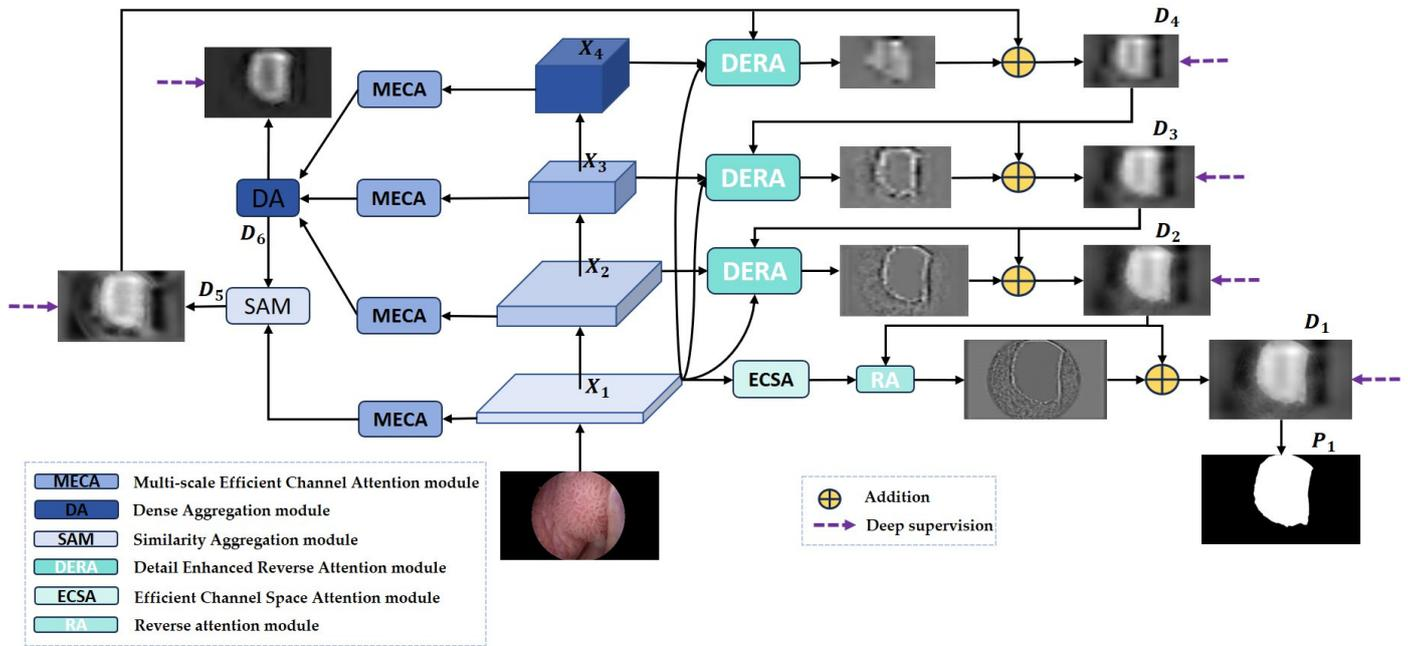
**Figure 2.** The architecture of the proposed MDER-Net, which consists of the backbone PVT v2, the multi-scale effective channel attention module (MECA), the dense aggregation module (DA), the similarity aggregation module (SAM), the detail-enhanced reverse attention module (DERA), the efficient channel space attention module (ECSA), and the reverse attention module (RA).
