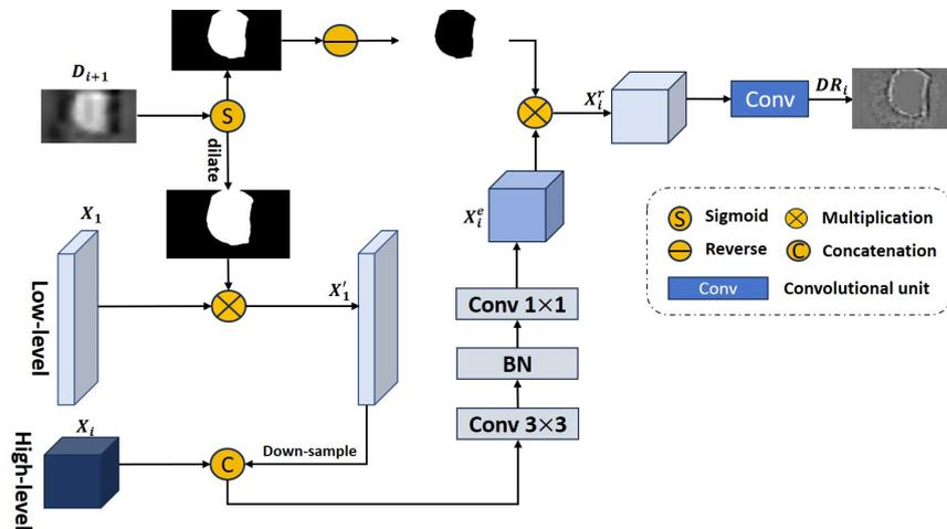
Figure 4. Structure of the proposed detail-enhanced reverse attention module (DERA).
