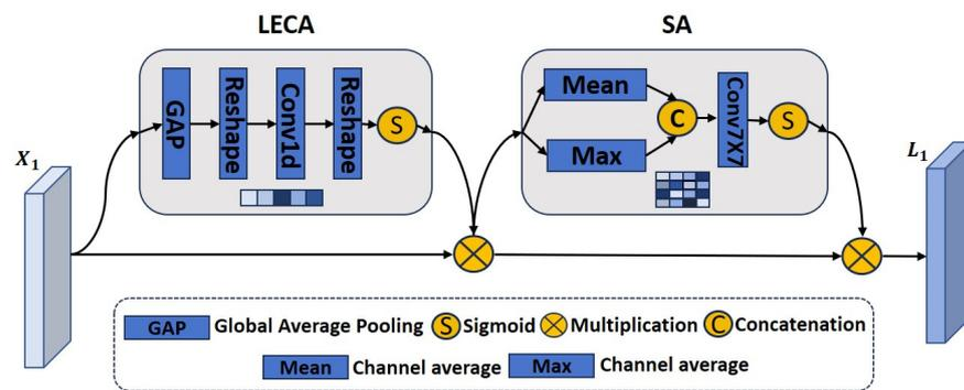
Figure 5. Structure of the proposed efficient channel space attention module (ECSA).
