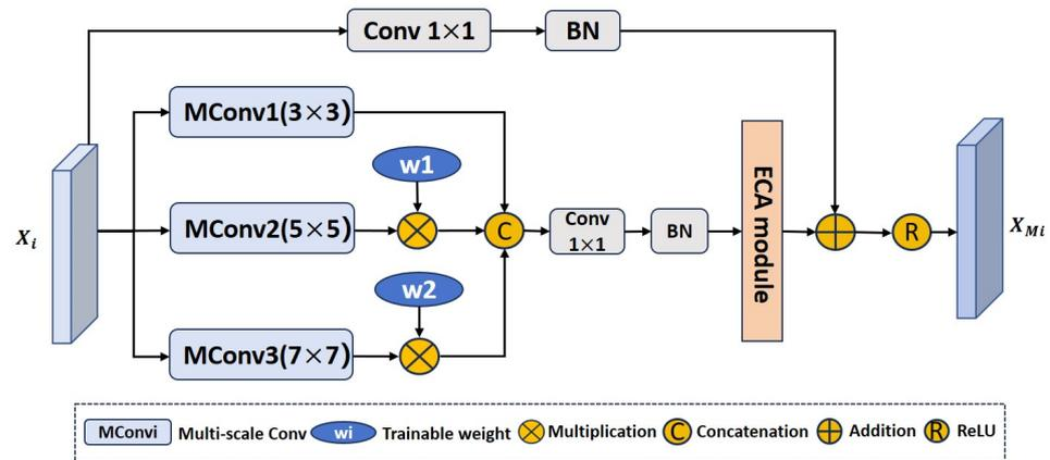
Figure 3. Structure of the proposed multi-scale efficient channel attention module (MECA).
