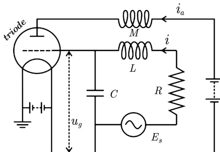
**Figure 5.** Electrical circuit involving a triode, resulting in a forced van der Pol oscillator.
