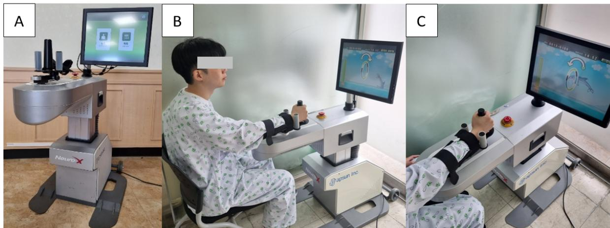
**Figure 2.** Robot-assisted upper-extremity training system (Neuro-X; Apsun, South Korea). (A). A 17-inch color touch screen monitor, base for upper-extremity exercise, and main body. (B,C). Patient sitting on a chair and training the paralyzed upper-extremity.
