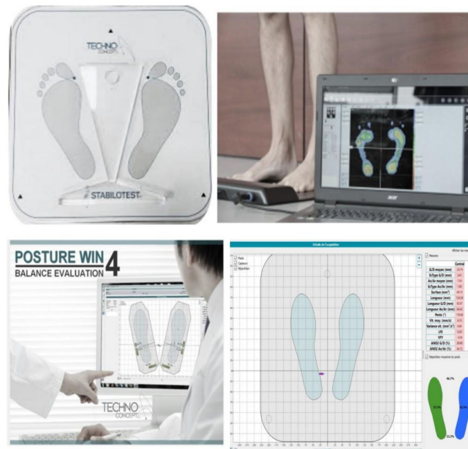
Figure 2. Stabilometric force platform (posture Win© 4).
