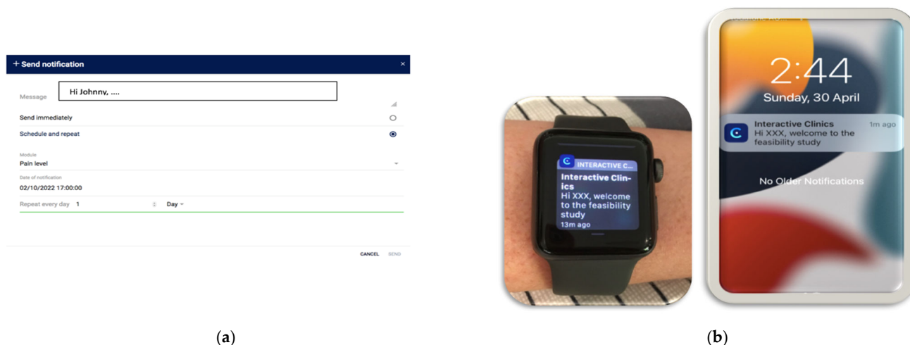
Figure 1. InteractiveClinics personalised automatic notification system. (a) Setting up personalised notifications on the web-based platform. (b) Notifications sent to the smartwatch and phone.
