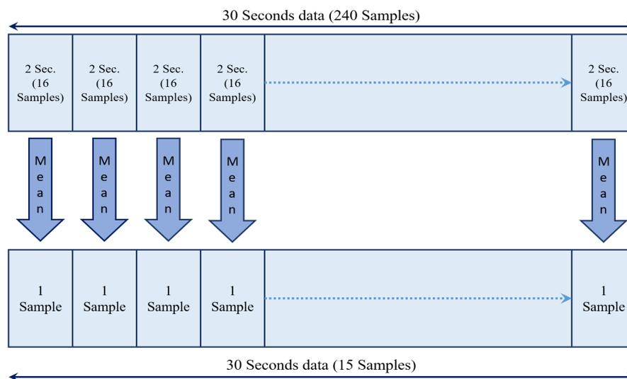
**Figure 4.** Schematic of the approach of segmentation.
