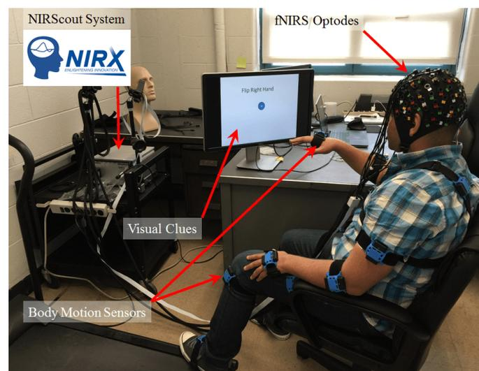
**Figure 3.** Experiment setup showing the sensors that has been used.
