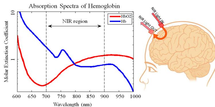
**Figure 1.** A schematic of how the fNIRS works with the absorption spectra of HbO<sub>2</sub> and Hb.
