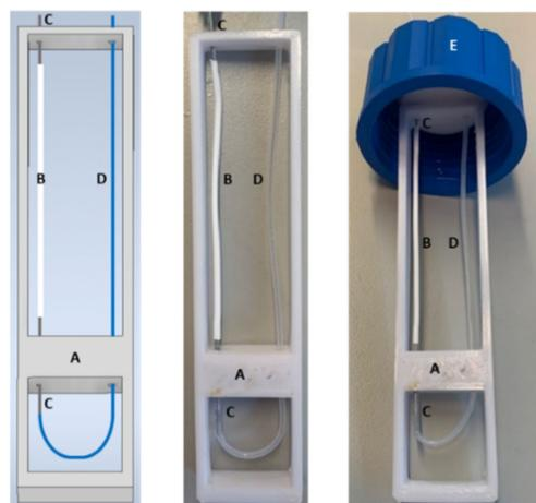
**Figure 2.** Support pictures of the microporous tube either designed by CAD (left) or manufactured in ABS by 3D printing. A: 3D support of the microporous tube; B: microporous tube of 7 cm long; C: bevelled stainless-steel tube serving as a connector for the microporous tube; D: 1/16-inch Teflon tube; E: GL 45 bottle cap.
