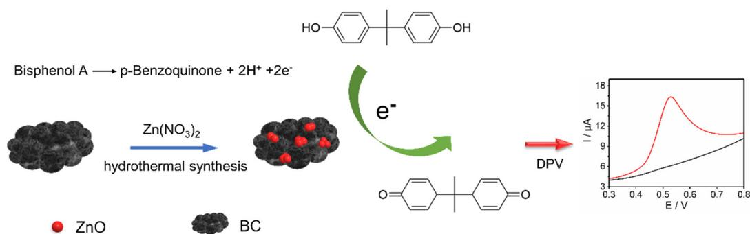
**Scheme 1.** The oxidation mechanism of BPA on ZnO/BC sensor.
