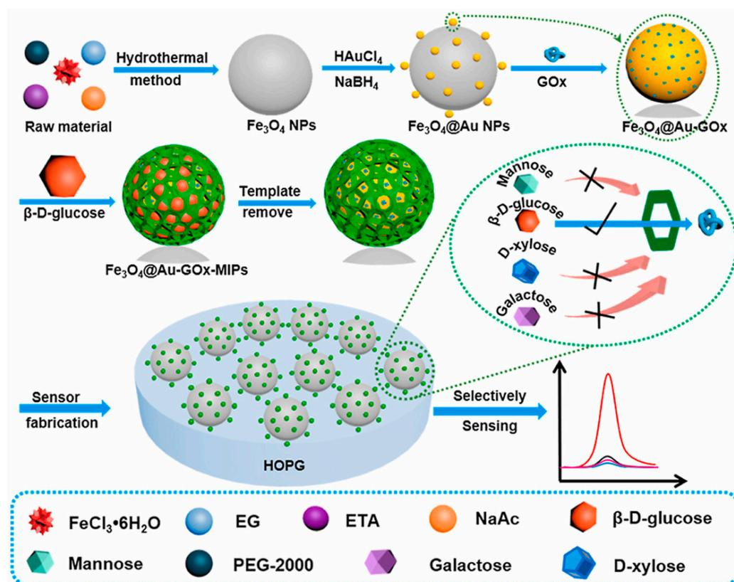
**Figure 7.** Preparation of the  $\text{Fe}_3\text{O}_4@Au\text{-GOx-MIPs}$  sensor and representation of the sensing mechanism achieved with CV analysis. Figure reproduced with permission from ref. [120]. Copyright 2022, Elsevier.
