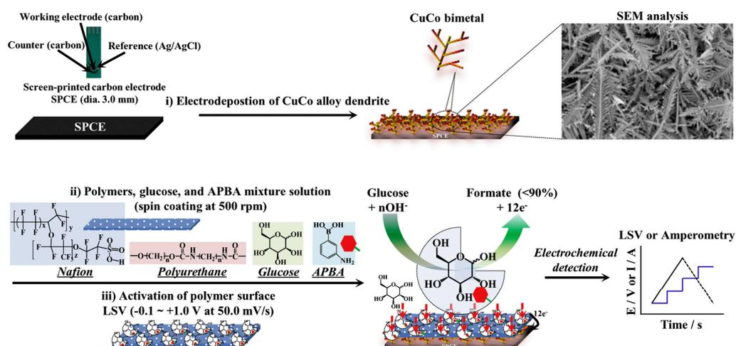
**Figure 6.** Representation of the glucose-imprinted polymer preparation and the two electrochemical readouts employed for the binding studies. Figure reproduced with permission from ref. [105]. Copyright 2018, Elsevier.
