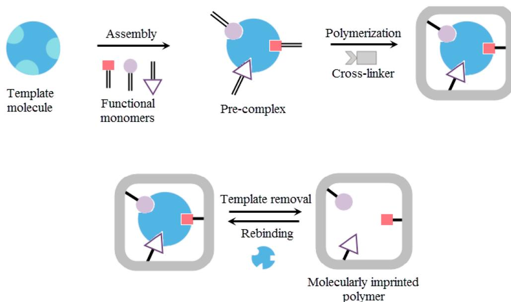
**Figure 2.** Schematic representation of generic synthesis and rebinding of molecularly imprinted polymers. Figure reproduced with permission from ref. [40].
