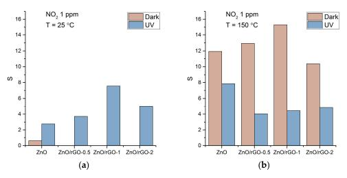
**Figure 10.** Sensor response of ZnO and ZnO/rGO composites when detecting 1 ppm NO<sub>2</sub> in dark conditions and under UV illumination at 25  $^{\circ}$ C (**a**) and 150  $^{\circ}$ C (**b**).
