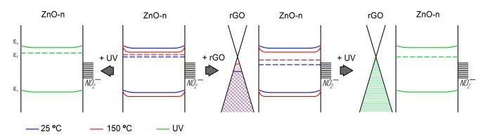
**Figure 9.** Scheme of ZnO band bending and ZnO/rGO heterojunction depending on temperature and UV illumination.
