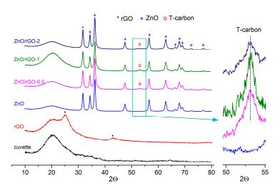
Figure 1. XRD patterns of rGO, ZnO, and ZnO/rGO nanocomposites with different rGO content.
