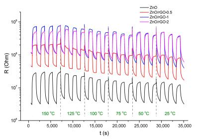
**Figure 6.** Dynamic change in sensors' resistance with periodic changes in the gas phase composition when detecting 1 ppm  $NO_2$  in dry air in the temperature range of 150–25 °C under UV illumination.
