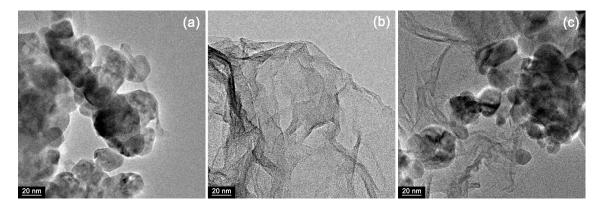
Figure 3. TEM images of ZnO nanofibers (a), rGO (b) and ZnO/rGO nanocomposite (c).
