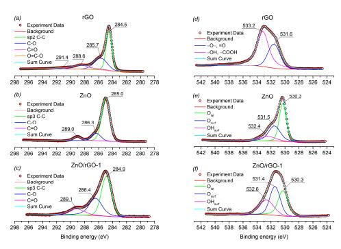
**Figure 5.** XP-spectra in C1s (**a**–**c**) and O1s (**d**–**f**) regions of rGO nanosheets (**a**,**d**), ZnO nanofibers (**b**,**e**) and ZnO/rGO-1 nanocomposite (**c**,**f**).
