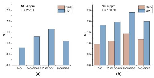
**Figure 11.** Sensor response of ZnO and ZnO/rGO composites when detecting 4 ppm NO in dark conditions and under UV illumination at 25  $^{\circ}$ C (**a**) and 150  $^{\circ}$ C (**b**).
