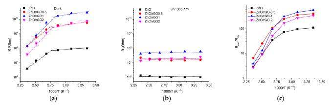
**Figure 8.** Temperature dependences of the resistance of ZnO nanofibers and ZnO/rGO composites: (a) In dark conditions; (b) Under constant UV illumination (365 nm). (c) Temperature dependences of  $R_{\text{dark}}/R_{\text{UV}}$  ratio.
