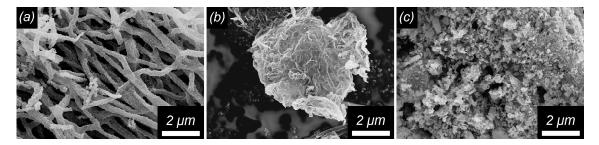
Figure 2. SEM images of ZnO nanofibers (a), rGO (b) and ZnO/rGO nanocomposite (c).
