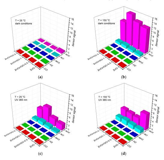
**Figure 7.** Sensor signal of ZnO nanofibers and ZnO/rGO composites when detecting reducing gases CO, NH<sub>3</sub>, H<sub>2</sub> and oxidizing gases NO and NO<sub>2</sub> in dark conditions (**a**,**b**) and under constant UV illumination (**c**,**d**) at  $T = 25 \,^{\circ}\text{C}$  (**a**,**c**) and  $T = 150 \,^{\circ}\text{C}$  (**b**,**d**).
