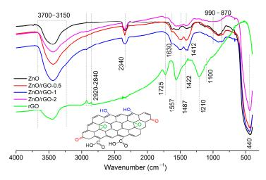
Figure 4. FTIR spectra of rGO, ZnO nanofibers, and ZnO/rGO nanocomposites.
