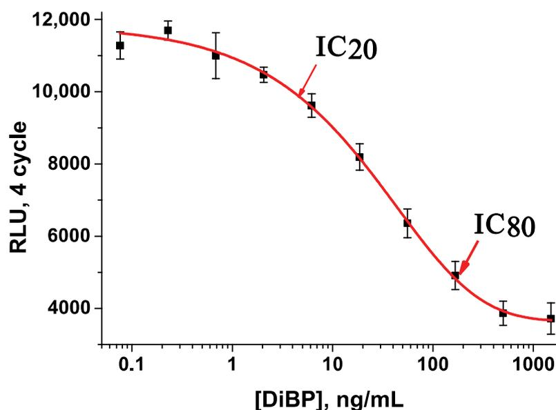
**Figure 5.** Calibration curve of CL-ELISA for the determination of DiBP using PBST buffer with 20% CH<sub>3</sub>OH, cycle 4 ( $R^2 = 0.995$ ).
