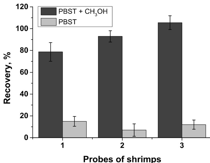
**Figure 6.** A histogram showing the average values of the detected DiBP in shrimp samples when extrapolating the data of relative luminescence units to the corresponding curve in PBST and PBST with methanol at the fourth measurement cycle. The values of DiBP in the case of methanol extraction were statistically significantly higher for all samples ( $n = 3$ ,  $p < 0.001$ ).
