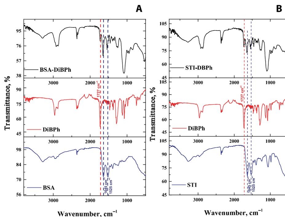
**Figure 2.** Characterization of BSA-DiBP (A) and STI-DiBP (B) by FT-IR technique, including spectra of corresponding conjugates (black lines), native DiBP (red lines), and native carrier proteins (purple lines).
