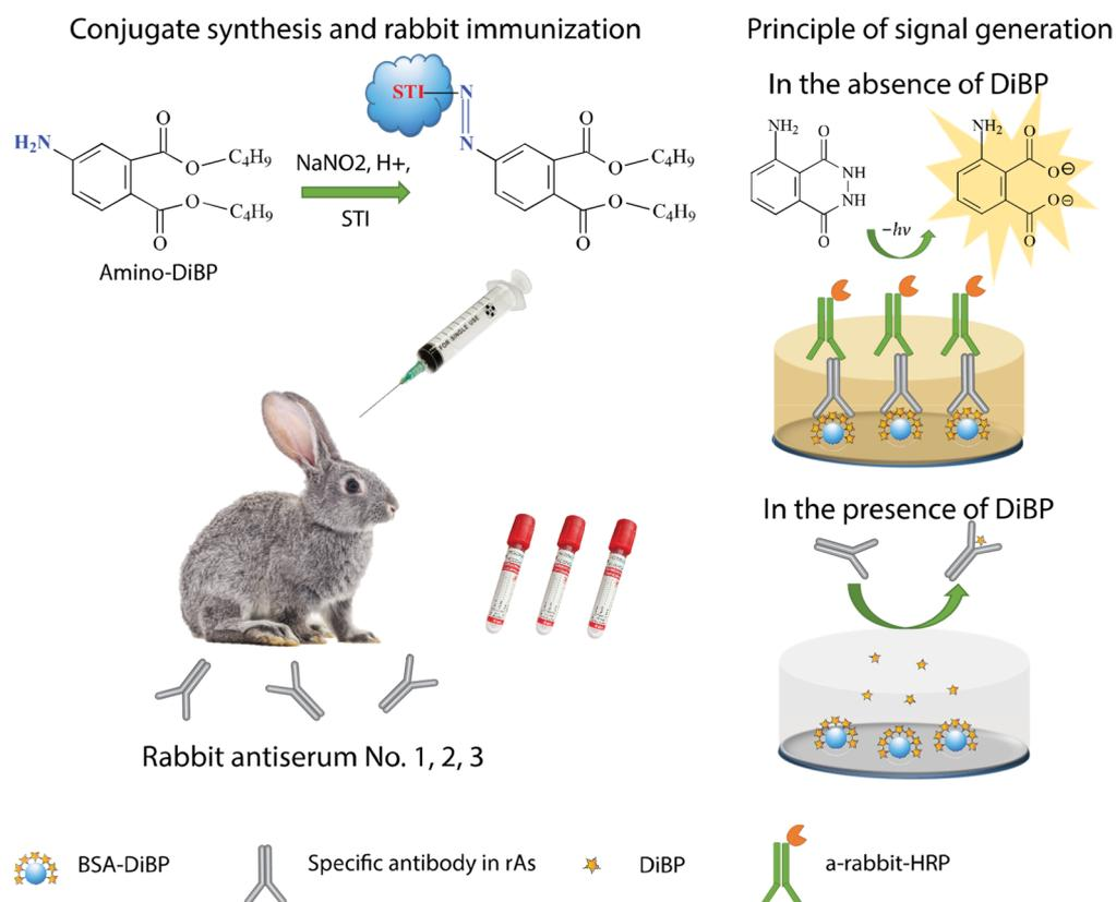
**Figure 1.** Principle of the proposed development, including two parts—immunization and the use of obtained antibodies. The left part demonstrates conjugate's synthesis by azo coupling method, rabbit immunization, and the obtaining of specific antibodies to DiBP. The right part shows the principle of the immune complexes formation and the generation of a chemiluminescent signal during the oxidation of luminol by horseradish peroxidase in microplate wells.
