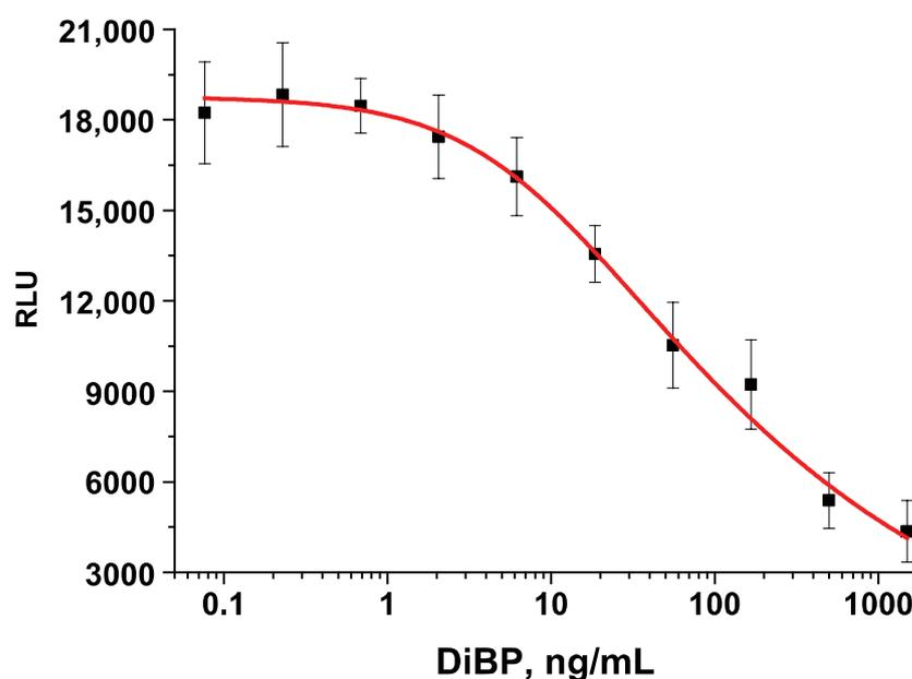
**Figure 4.** Dependence of the chemiluminescent signal on the DiBP concentration in PBST ( $n = 2$ ), cycle 1 ( $R^2 = 0.991$ ).
