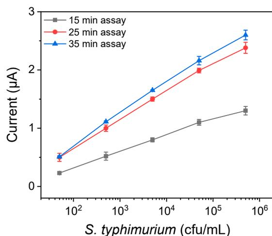
**Figure 4.** *S. typhimurium* calibration curves obtained for total assay time of 15 min (black line), 25 min (red line), and 35 min (blue line).
