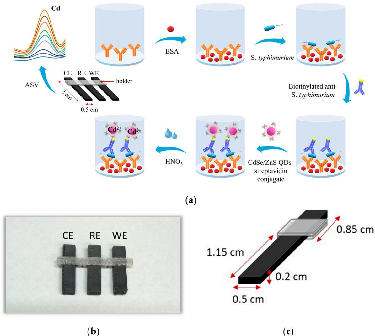
**Figure 1.** (a) Schematic of *S. typhimurium* immunoassay steps. (b) Image of the 3D-printed electrochemical sensor. (c) Schematic of the electrode along with the holder indicating their dimensions.
