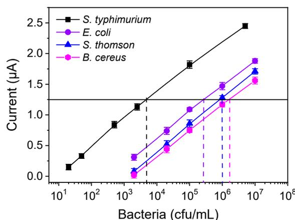
**Figure 7.** Calibration curves of *S. typhimurium*, *S. Thomson*, *E. coli*, and *B. cereus* in assay buffer. Each point corresponds to the mean value of four different measurements. Error bars represent  $\pm$ SD.
