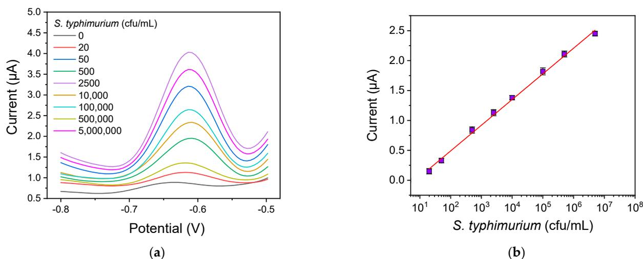
**Figure 6.** (a) Voltammograms obtained from different concentrations of *S. typhimurium* in assay buffer. (b) Calibration curve of *S. typhimurium* in assay buffer. Each point corresponds to the mean value of four different measurements. Error bars represent  $\pm SD$ .
