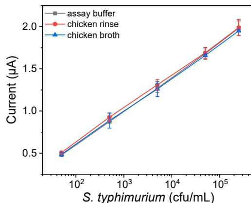
**Figure 5.** Calibration curves of *S. typhimurium* corresponding to net signals obtained for the different calibrators prepared in assay buffer (black line), chicken rinse (red line), and chicken broth (blue line) using the electrochemical immunosensor.
