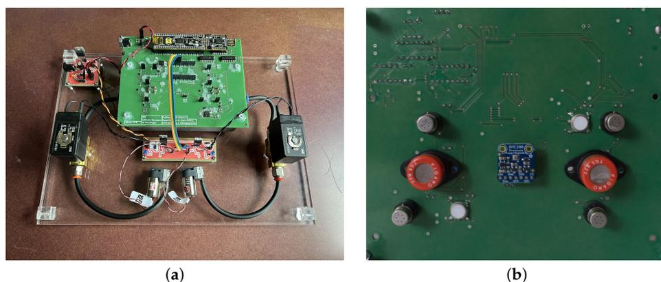
**Figure 2.** (a) Top view of the PCB integrating the circuit for TM of gas sensors, together with the associated components required for its functioning. (b) Bottom view of the temperature-modulated electronic nose, showing the gas sensors and the environmental sensor, located at the center of the board in contact with the analysis chamber.
