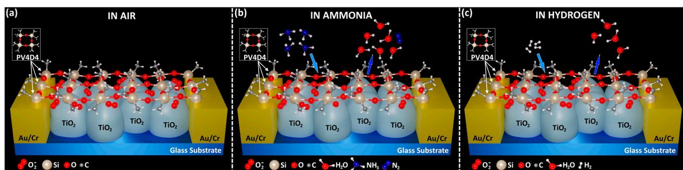
**Figure 9.** The proposed sensing mechanism of PV4D4-coated TiO<sub>2</sub> nanostructures (a) in air, (b) in ammonia, and (c) in hydrogen [117].
