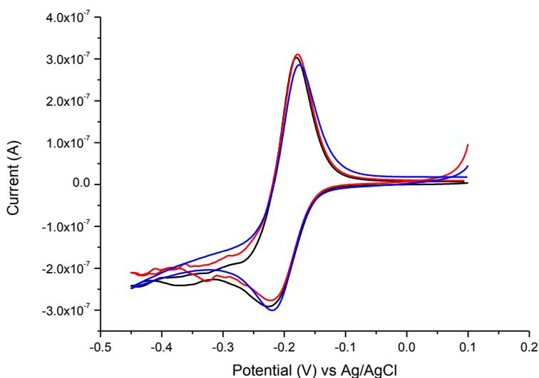
**Figure S1.** CVs of 0.1 mM MB in 0.01 M PBS recorded at three different bare NEEs. Scan rate: 10 mV/s.
