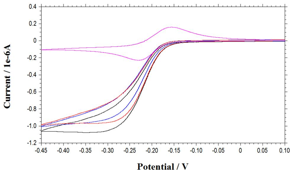
**Figure S2:** Cyclic voltammograms recorded at the NEE immunosensor in 0.1 mM MB, 0.01 M PBS solution; scan rate 10 mV/s. Black line 0.5 mM, red 1.0 mM and blue line 1.5 mM H<sub>2</sub>O<sub>2</sub>.
