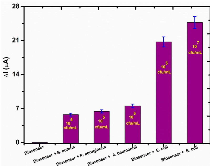
**Figure S7.** Change in the DPV current of the biosensor in the presence of different bacteria having a concentration of  $10^5$  CFU/mL. ( $\Delta I = (I_0 - I)$ , where  $I_0$  is the current of biosensor in the absence of bacteria and  $I$  is the current of the biosensor in the presence of bacteria.).
