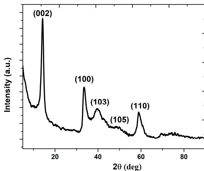
**Figure S1.** Powder XRD pattern of MoS<sub>2</sub> nanosheets.
