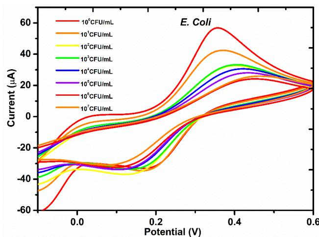
**Figure S6.** CV spectra of the biosensor in the presence of *E. coli* in 5 mM  $[\text{Fe}(\text{CN})_6]^{3-/4-}$ , 0.1 M KCl, and 0.1 M PBS buffer (pH = 7.4).
