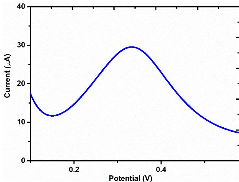
**Figure S8.** DPV spectra of the biosensor electrode after 21 days of storage at 4 °C in 5 mM [Fe (CN)<sub>6</sub>]<sup>3-/4-</sup>, 0.1 M KCl, and 0.1 M PBS buffer (pH = 7.4).
