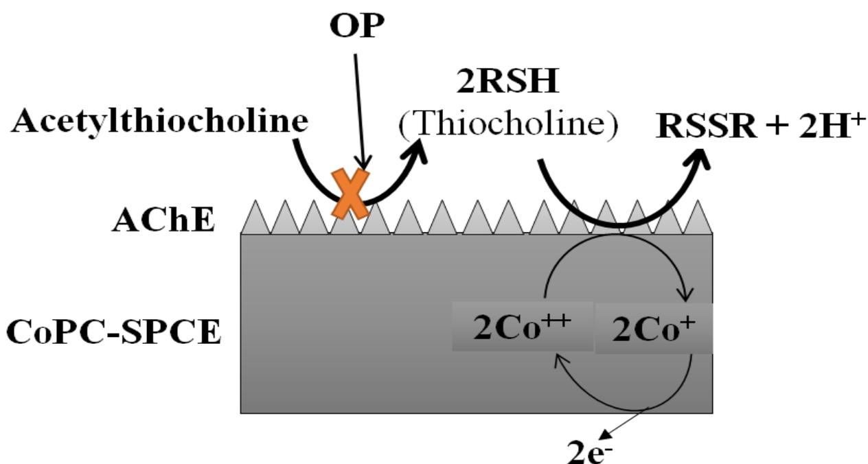
**Figure 7.** Schematic diagram explaining the principle of the reactions based on this amperometric biosensor. Adapted from Crew et al. [228].
