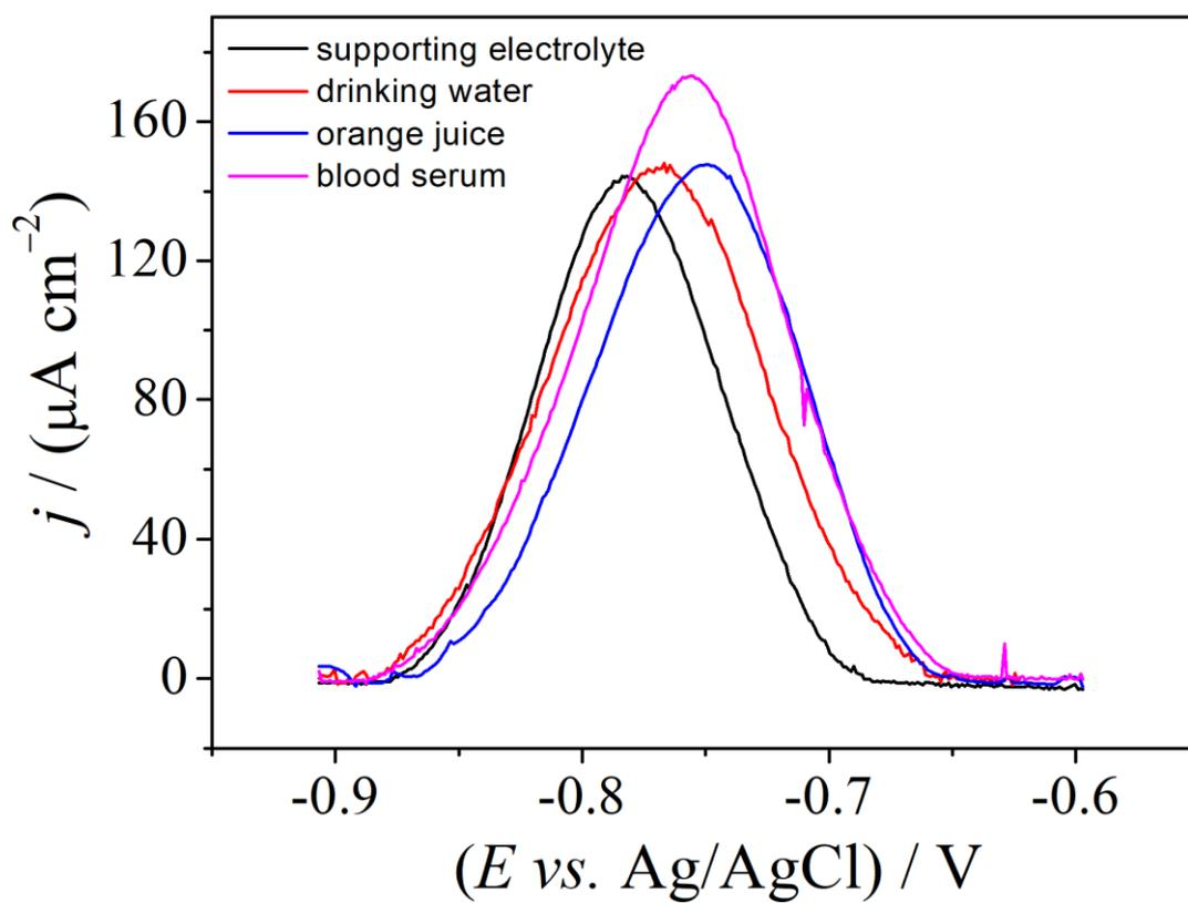
**Figure S6.** Square-wave voltammograms obtained for the quantification of paraquat in different matrices using the paper-based silver sensor. Supporting electrolyte:  $0.1 \text{ mol L}^{-1}$   $\text{Na}_2\text{SO}_4$  solution (pH 7.0). SWV conditions:  $f = 3 \text{ Hz}$ ;  $a = 60 \text{ mV}$ ;  $\Delta E = 2 \text{ mV}$ .
