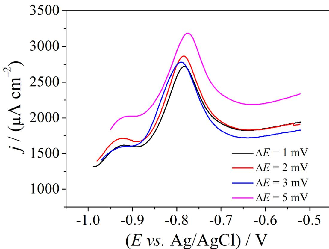
**Figure S4.** Square-wave voltammograms obtained as function of the scan increment variation using the paper-based silver sensor in the presence of  $100 \mu\text{mol L}^{-1}$  paraquat in  $0.1 \text{ mol L}^{-1} \text{Na}_2\text{SO}_4$  solution (pH 7.0). SWV conditions:  $f = 3 \text{ Hz}$ ;  $a = 60 \text{ mV}$ .
