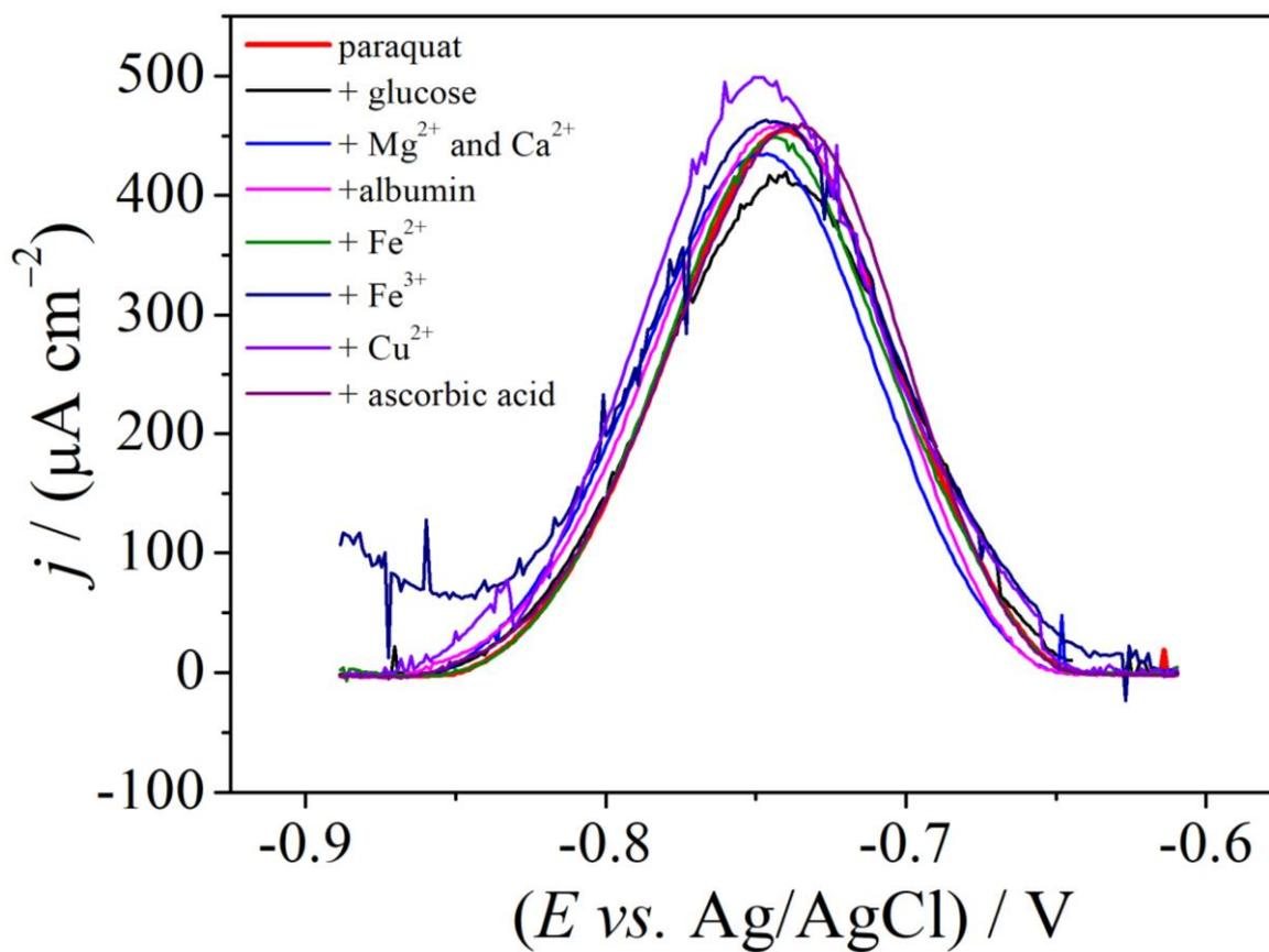
**Figure S5.** Square-wave voltammograms obtained using the paper-based silver sensor for  $50 \mu\text{mol L}^{-1}$  paraquat in  $0.1 \text{ mol L}^{-1}$   $\text{Na}_2\text{SO}_4$  solution (pH 7.0) in the presence of possible interferents. SWV conditions:  $f = 3 \text{ Hz}$ ;  $a = 60 \text{ mV}$ ;  $\Delta E = 2 \text{ mV}$ .
