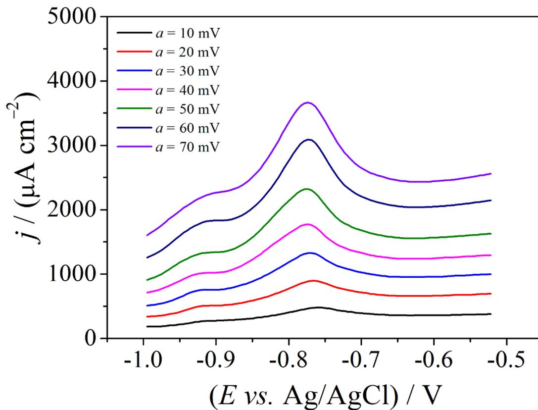
**Figure S3.** Square-wave voltammograms obtained as function of the pulse amplitude variation using the paper-based silver sensor in the presence of  $100 \mu\text{mol L}^{-1}$  paraquat in  $0.1 \text{ mol L}^{-1} \text{Na}_2\text{SO}_4$  solution (pH 7.0). SWV conditions:  $f = 3 \text{ Hz}$ ;  $\Delta E = 5 \text{ mV}$ .
