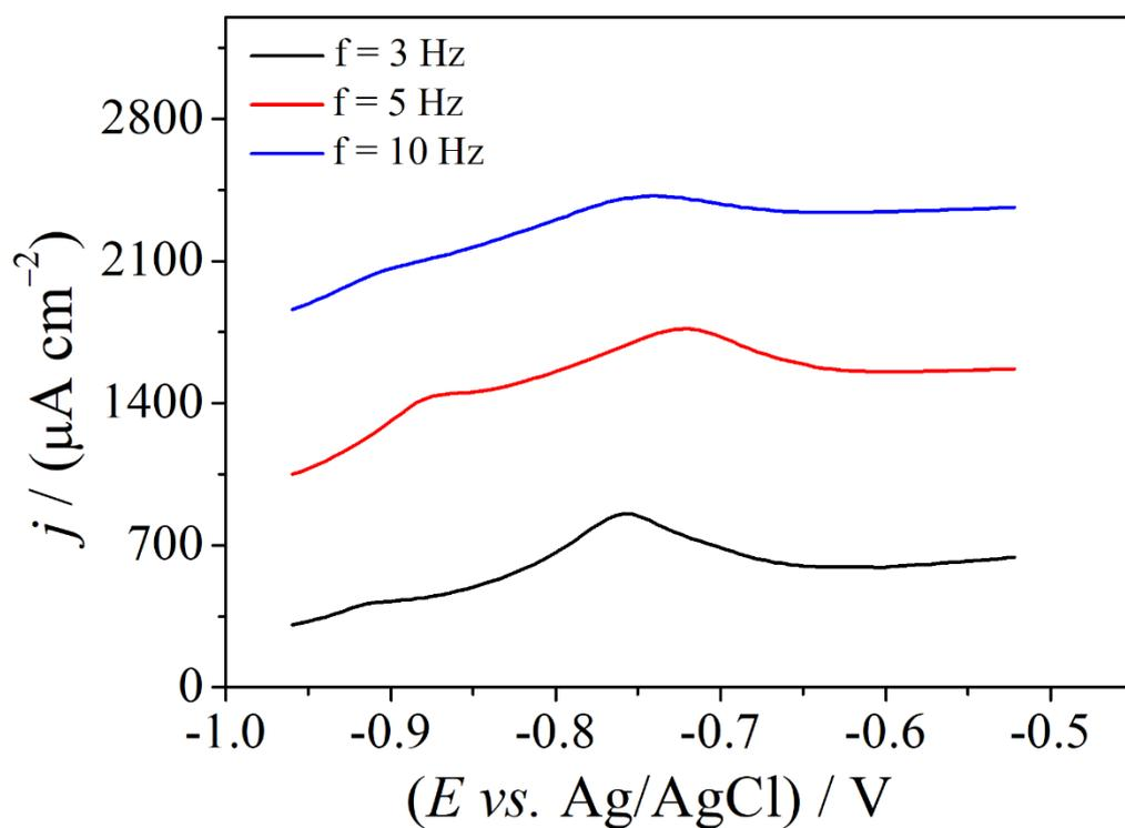
**Figure S2.** Square-wave voltammograms obtained as function of the square-wave frequency variation using the paper-based silver sensor in the presence of  $100 \mu\text{mol L}^{-1}$  paraquat in  $0.1 \text{ mol L}^{-1} \text{ Na}_2\text{SO}_4$  solution (pH 7.0). SWV conditions:  $a = 20 \text{ mV}$ ;  $\Delta E = 5 \text{ mV}$ .
