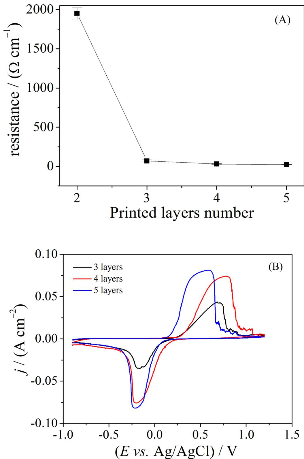
**Figure S1.** (A) Resistance of paper-based inkjet-printed electrode and (B) Cyclic voltammograms of silver electrode in 0.5 mol L<sup>-1</sup> H<sub>2</sub>SO<sub>4</sub> solution as function of printed layers number.
