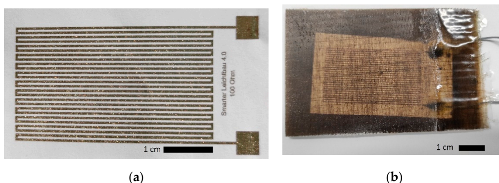
Figure 4. (a) Printed temperature sensor on the paper substrate; (b) bottom view of integrated sensor sample.
